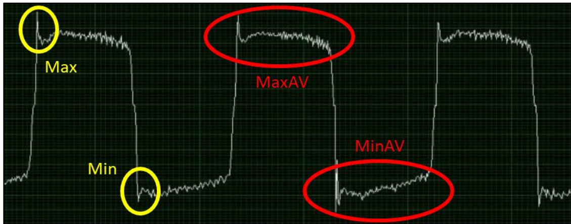
Figure 2.5: 5 An output voltage trace from the pin-on-plate rig highlighting regions where voltage measurements were taken, maximum and minimum voltages (yellow circles), maximum average and minimum average voltage (red ovals).
