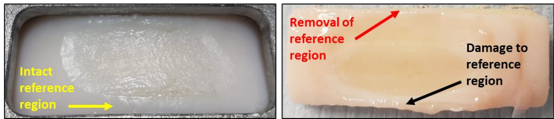
Figure 3.20: Plate sample showing a suitable area outside of the contact region (yellow arrow) to use a reference (left). Plate sample with extensive damage leaving no suitable reference region due to removal (red arrow) or displacement of cartilage (right).
