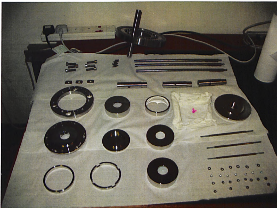
Figure 3.3: Electrostatic lens components. All components were machined from 316 stainless steel except for the mounting flange (304 grade stainless steel) and the ruby ball spacers.
