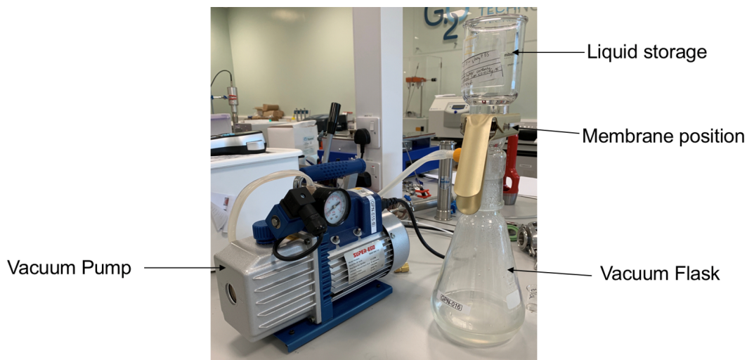
Figure 3.1: Labelled vacuum deposition experimental setup, showing the vacuum pump connected to a vacuum flask via tubing. GO dispersion is pipetted onto a secured PES membrane, and the liquid phase is pulled through the membrane pores, meanwhile a GO coating remains on the polymer surface.
