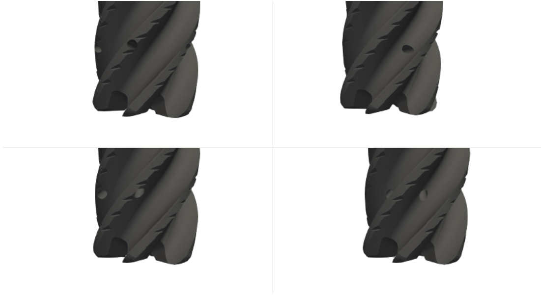
Figure 4.9: Extreme geometries (a) \theta_v = 0, \theta_h = 12.5 (b) \theta_v = 0, \theta_h = 55 (c) \theta_v = 45, \theta_h = 19 (d) \theta_v = 45, \theta_h = 37 .
