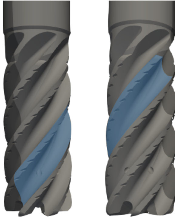
Figure 5.6: Views of the engaged region of a single flute (blue) from both sides of the tool. Dark grey colouring shows the disengaged regions of the tool, with light grey showing the engaged regions. The blue coloured single flute spans the height of the tool and can not be seen in entirety from a single perspective.
