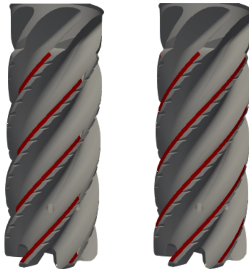
Figure 5.5: Engaged cutting edges of the tool for side milling operations (left) with lower radial engagements, and full slot milling (right) with total radial engagement.
