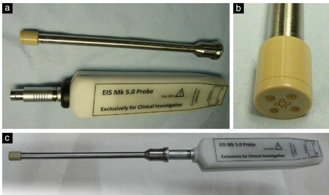
Figure 3.1: The EIS device of Sheffield Mark V, showing the device base, and the device probe piece (a), the tetrapolar probe configuration (b) and the complete coupled device (c).
