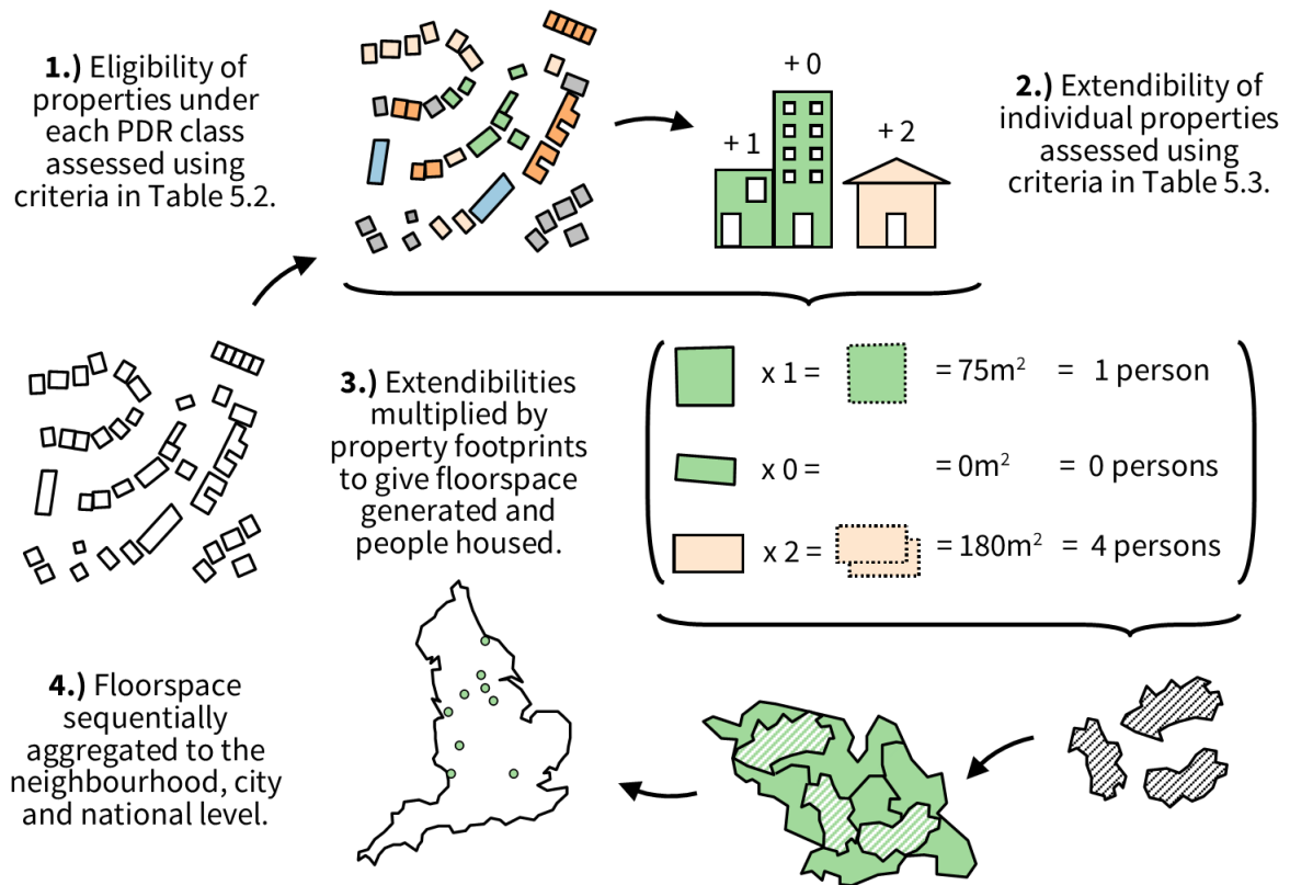
Figure 5.1 - Overview of the developed bottom-up assessment framework. Further details may be found in Section 5.3.3.
