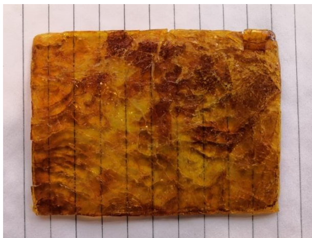
Figure 55: Inhomogeneous compression moulded plate of 40AEMA20 cross-linked with 10 mol.% of DAM2
