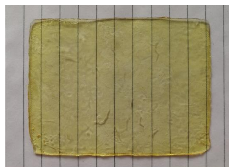
Figure 54: The structure of Priamine™ 1075 ( DAM2 ) (left) and a picture of a typical cross-linked network obtained from poly(EHMA-co-AEMA) cross-linked with DAM2 (right).
