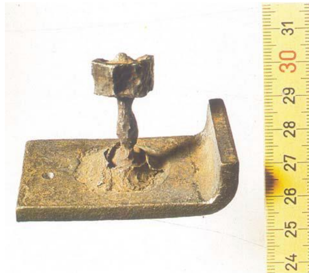
Figure 2.54: The formation of galvanic corrosion is found in a ray lamp of a distillation column which occurred at the interface between a stainless steel AISI 410 plate in contact with a carbon steel bolt in an environment with hydrocarbons contaminated with salts [116].
