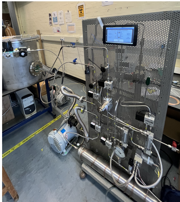
Figure 6.9 Photo of gas system prototype connected to a 100L test vessel.
