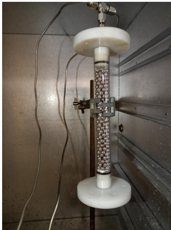
Figure 3. 12 - Image of the longer bead pack of 150mm height in the oven.
