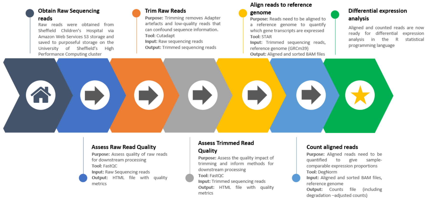
Figure 5-8: Workflow for RNA-Sequencing pre-processing. Briefly, raw reads are obtained from the sequencing facility and transferred to a high-performance computing environment. These raw reads are subsequently checked for quality, trimmed and quality reassessed post-trimming, before being aligned to a reference genome and subsequently quantification of aligned reads leads to a counts file output that is used in assessment of differential gene expression and further downstream processing.
