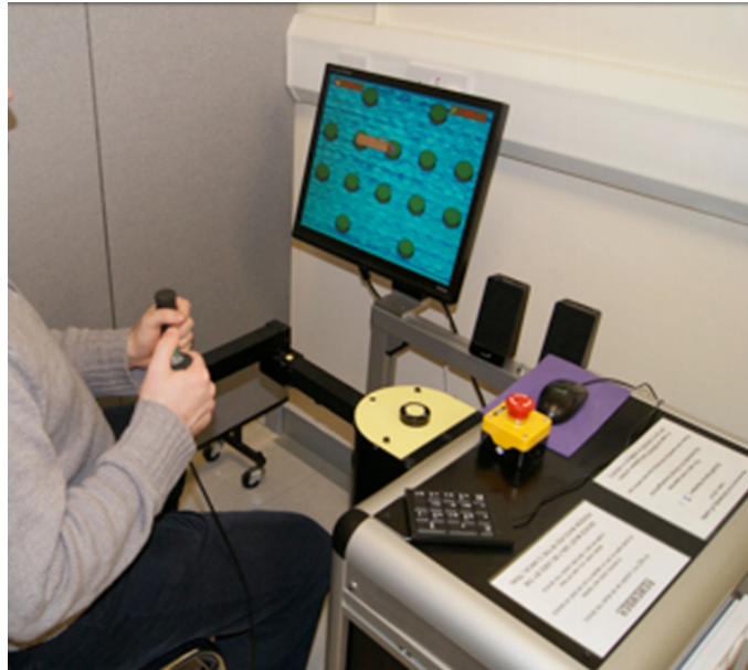
Figure 2.15: The hCAAR System Assisting a User to Reach Targets Presented by a Screen [11].
