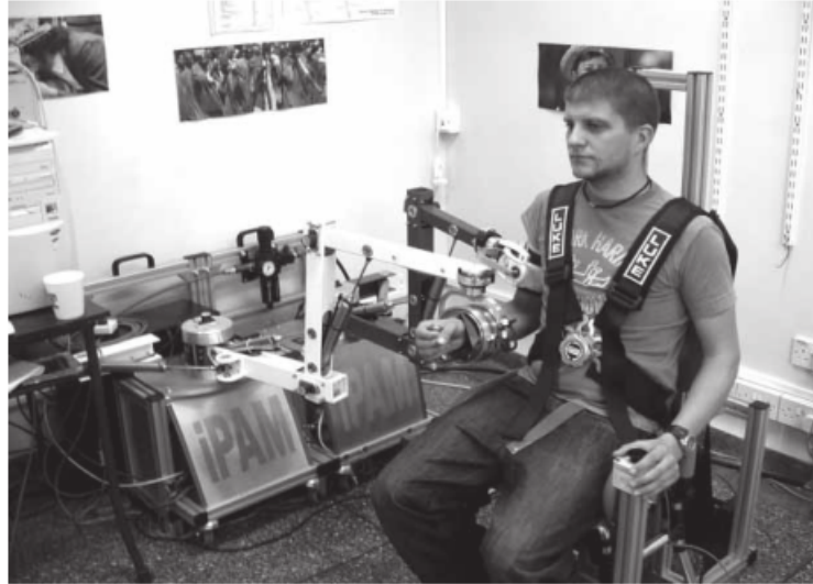
Figure 2.14: The iPAM System [80], Showing the Cooperative Dual Robots Guiding a User's Arm.
