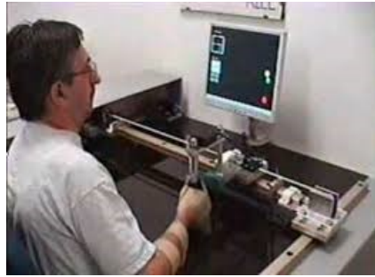
Figure 2.10: The MEMOS System Assisting a User to Reach Targets Presented on a Screen [72].
