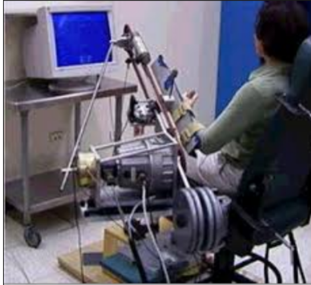
Figure 2.12: The ARM Guide System Assisting a User to Reach Targets presented on a Screen [76].
