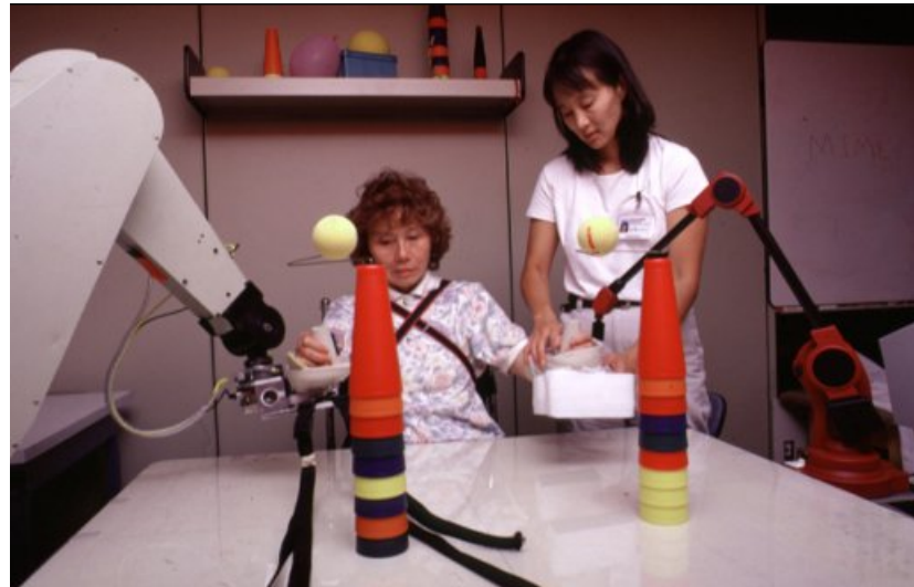
Figure 2.11: The 3rd Iteration of the MIME System Assisting a User to Perform Reaching exercises [39].
