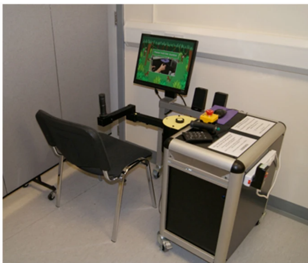
Figure 1.2: The hCAAR Rehabilitation Robot [11], Which Had a Much Larger Footprint Than the Current Iteration of MyPAM.
