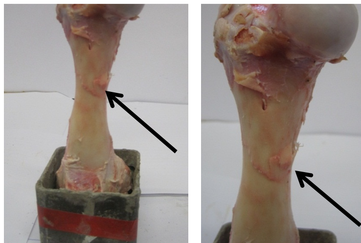
Figure 5.13. A single sample tested to destruction under compressive loading. As can be seen, fracture of the sample has occurred beneath the femoral head, along the medial face.
