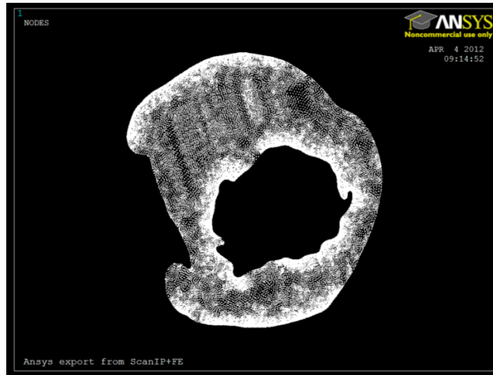
Figure 7.5. Nodal plot of the upper face of a cropped sample of cortex. The medial aspect (uppermost) and posterior aspect (left) show thicker walls, providing complication during the application of distributed loading.
