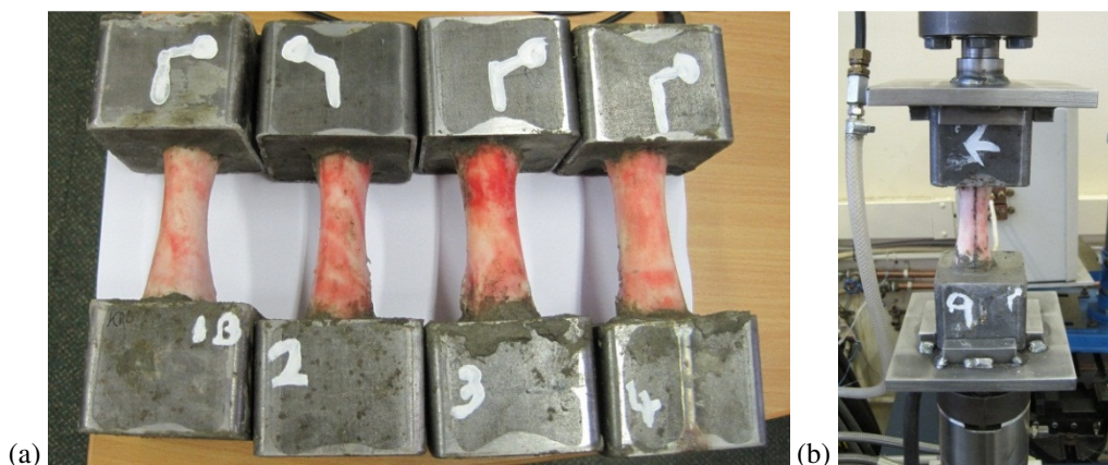
Figure 5.3. (a), A selection of potted samples for testing - clear differences in bone geometry can be noted. (b) A sample prior to testing with the direction of force application clearly indicated on the upper constraint.
