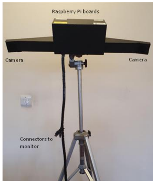
Figure 2.3 BIGKAT camera system as seen from the participant's view
