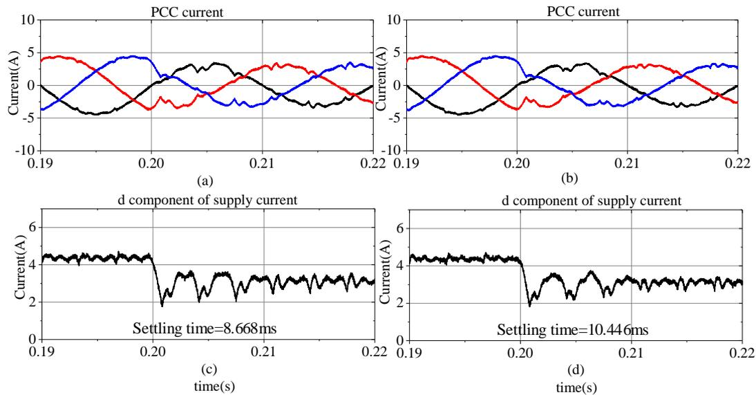
Figure 2.28: The variations of the current waveforms using the method with data expansion: The  $I_S$  (a) from period 3 to period 4 when the maximum number of notch filters is 4 (b) when the maximum number is 5. The  $I_{Sd}$  (c) from period 3 to period 4 when the maximum number of notch filters is 4 (d) when the maximum number is 5.
