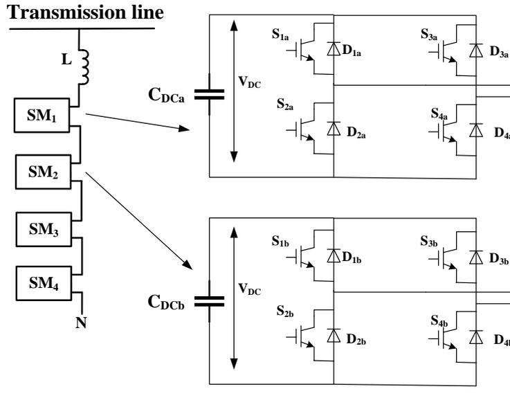
Figure 1.25: The configuration of 9-level CHB
