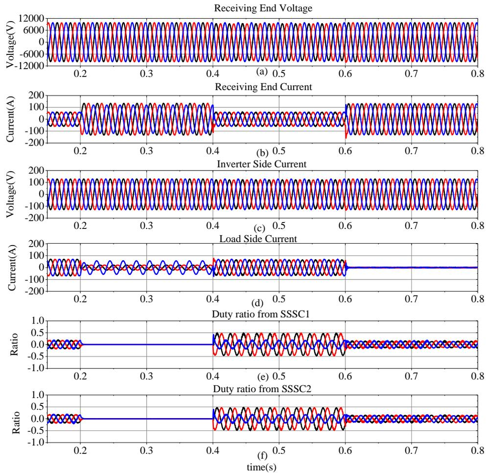
Figure 5.16: Scenario 3: the measured waveforms (a) the receiving end voltages, (b) the receiving end current, (c) the load side current, (d) the DG side current, (e) the duty ratio for the SSSC1 and for (f) the SSSC2.
