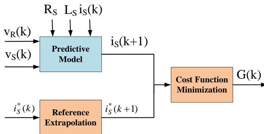
Figure 3.6: The control block diagram of the OSS-MPC
