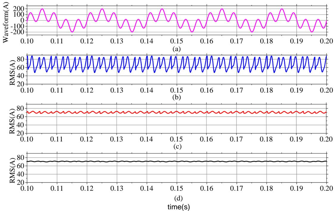
Figure 2.13: (a) The Original signal waveform. The RMS values of the 5th order element in the reconstructed signal by (b) db8, (c) db30, (d) discrete meyer.
