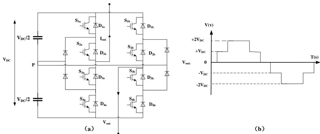
Figure 1.24: (a) Five-level Neutral Point Clamped Converter (NPC) circuit (b) Voltage level
