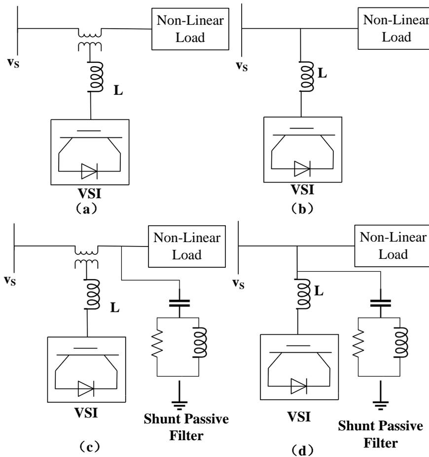
Figure 2.2: The configurations of (a) series APF, (b) shunt APF, Hybrid APF
