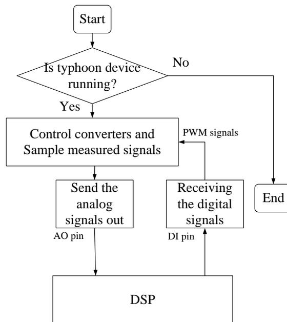
Figure 4.9: The flow chart of the operation stage for the typhoon HIL device
