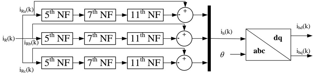
Figure 2.9: The control diagram of the notch filter-based extraction method
