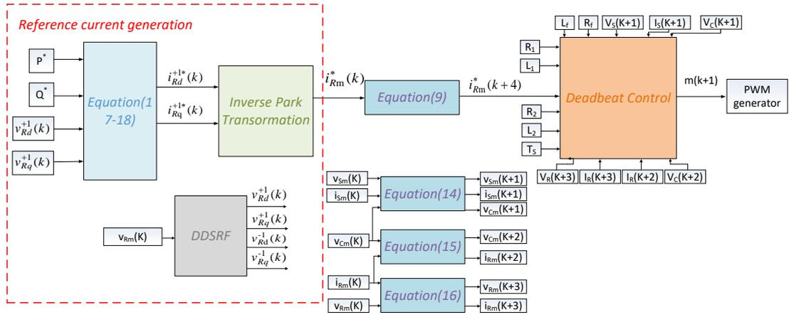
Figure 4.5: The overall control strategy of the transformerless-SSSC
