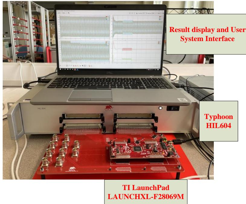
Figure 4.7: The experimental set-up for the real-time DSP control of a Typhoon HIL 604 emulated power line with the TL-SSSC
