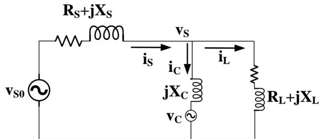
Figure 1.3: The equivalent circuit of STATCOM
