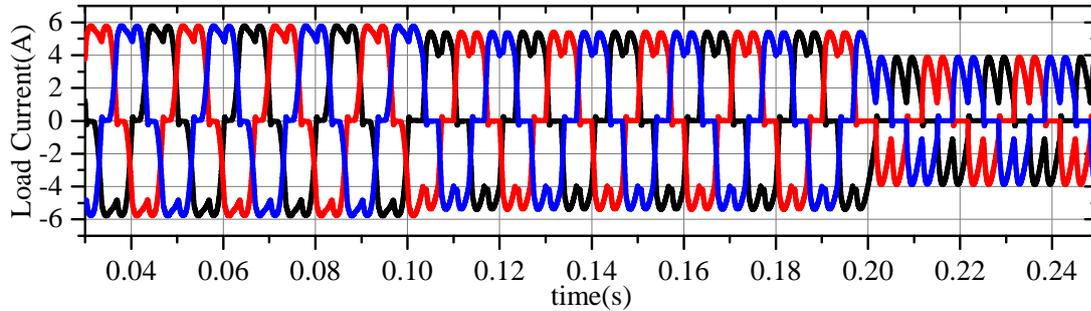
Figure 2.22: The load current  $I_R$  from the non-linear load when the firing angle changes from  $0^\circ$  to  $30^\circ$  at 0.1s and from  $30^\circ$  to  $45^\circ$  at 0.2s.
