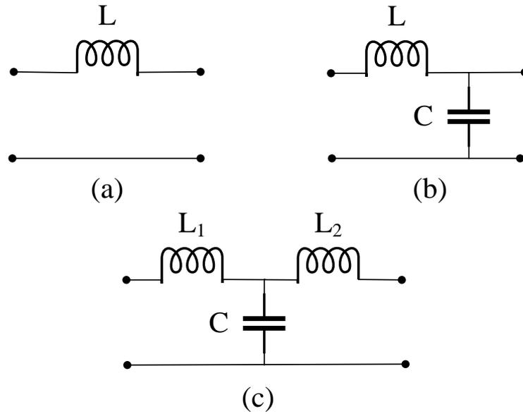
Figure 2.1: The passive power filters (a) L filter (b) LC filter (c) LCL filter
