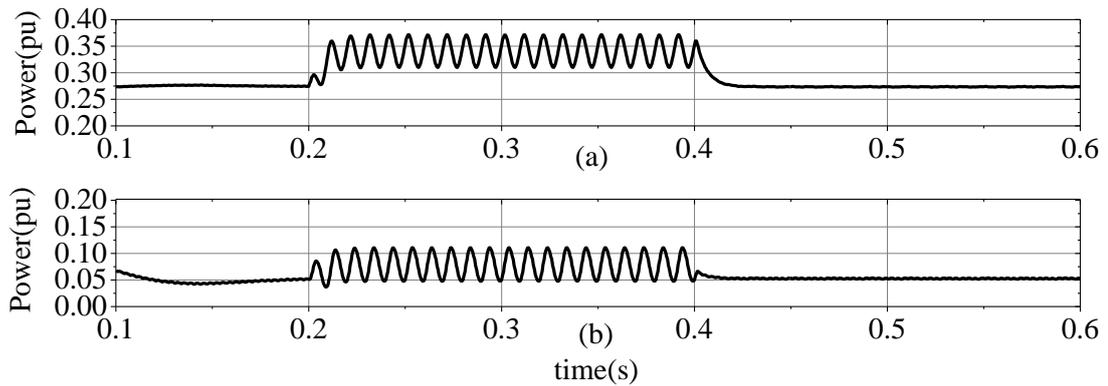
Figure 4.16: (a) The active power and (b) the reactive power at the grid sending end
