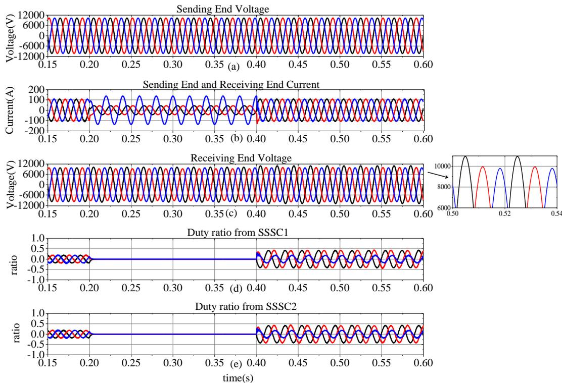
Figure 5.14: Scenario 2: the measured waveforms (a) the sending end voltages, (b) the sending end and receiving end currents, (c) the receiving end voltages, (d) the duty ratio for the SSSC1 and for (e) the SSSC2.
