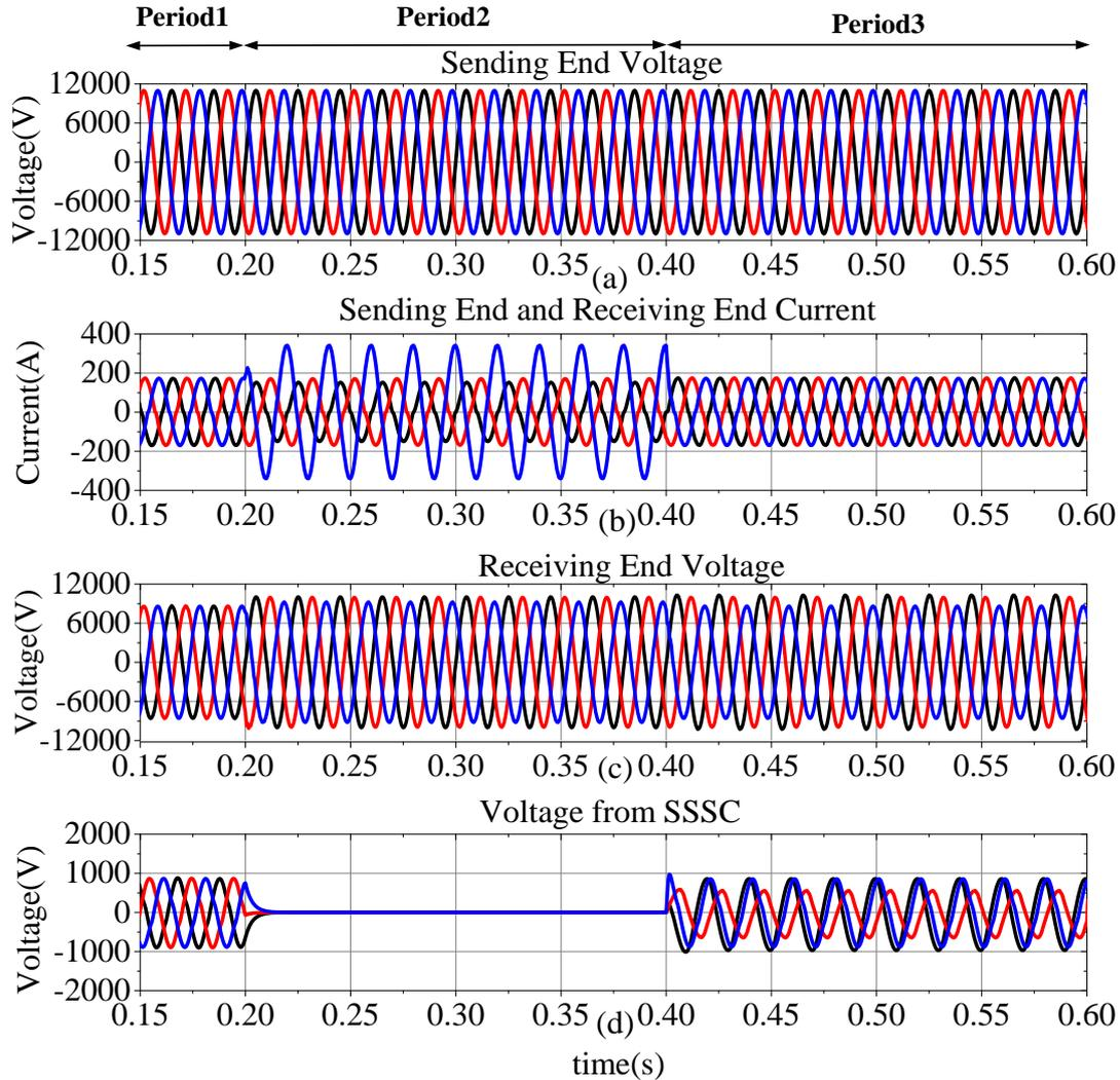
Figure 4.15: The measured waveforms from the proposed method for scenario 2 (a) the sending end voltages, (b) the sending end and receiving end currents (c) the receiving end voltages, (d) the TL-SSSC generated voltage
