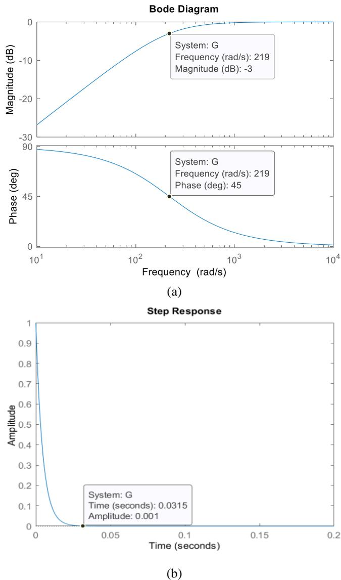
Figure 2.6: (a) The bode diagram and (b) the step response of a high pass filter when the cut-off frequency is 219.1 rad/s
