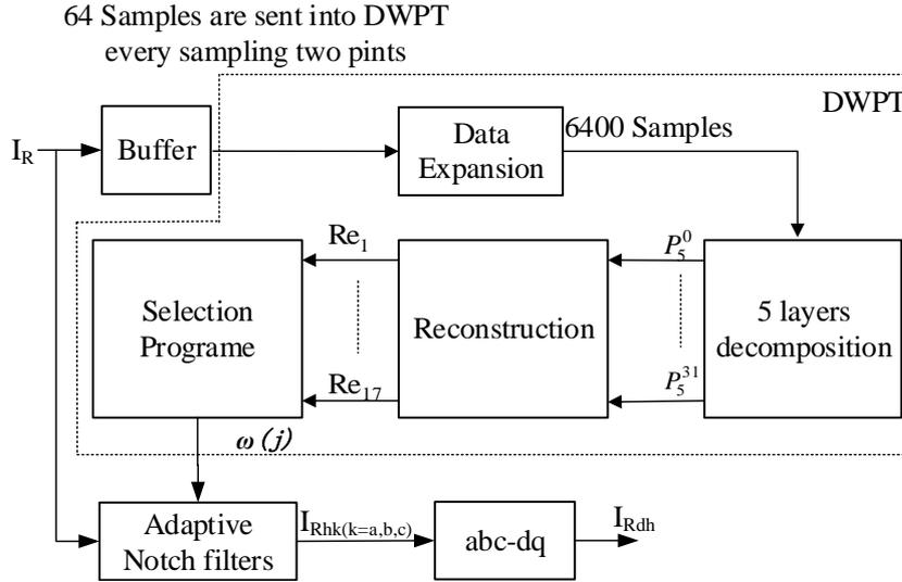
Figure 2.20: The schematic of the real-time DWPT harmonic identification.
