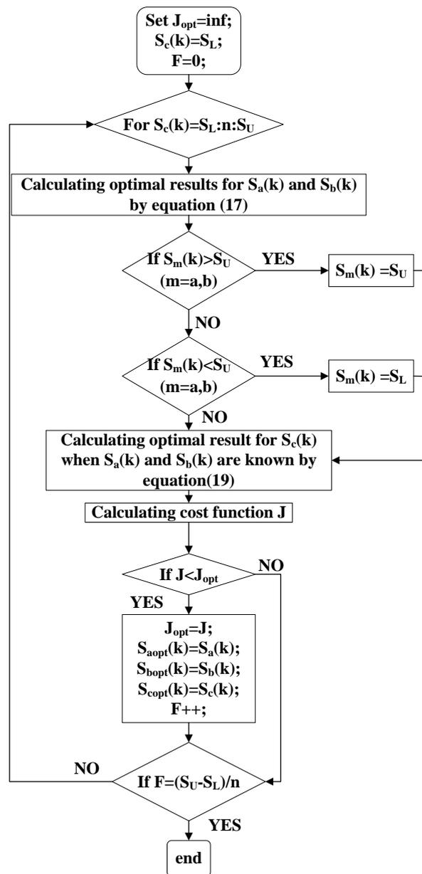
Figure 3.11: The flowchart for the modified branch and bound (B&B) method
