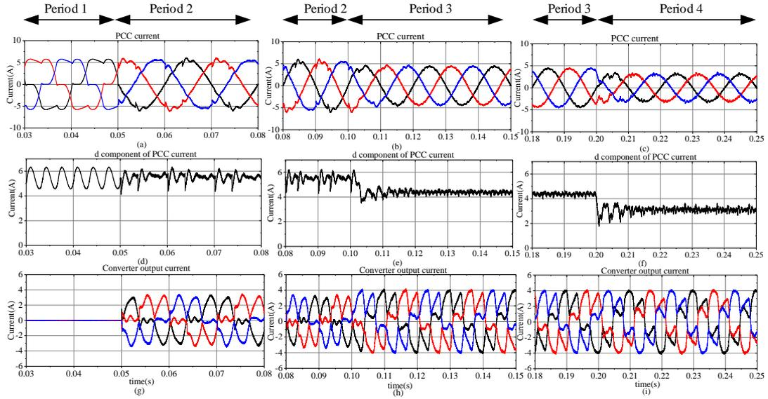
Figure 2.27: The variations of the current waveforms using the method without data expansion: The  $I_S$  (a) from period 1 to period 2 (b) from period 2 to period 3 (c) from period 3 to period 4. The  $I_{Sd}$  (d) from period 1 to period 2 (e) from period 2 to period 3 (f) from period 3 to period 4. The compensation current  $I_C$  (g) from period 1 to period 2 (h) from period 2 to period 3 (i) from period 3 to period 4
