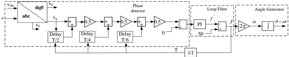
Figure 1.17: The control diagram of the CDSC-PLL
