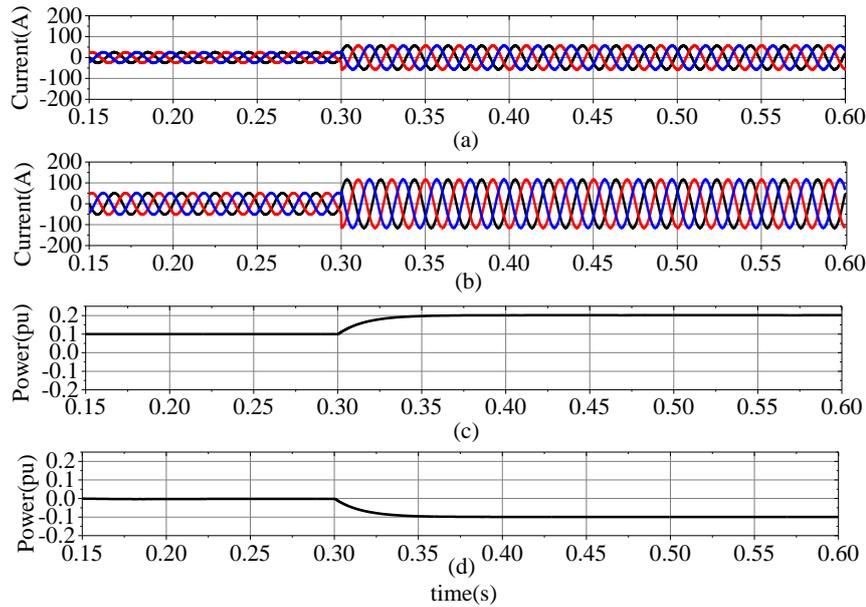
Figure 5.9: (a) The SSSC1 and the SSSC2 branch current (b) the receiving end current (c) the active power and (d) the reactive power at the receiving end for the balanced situation
