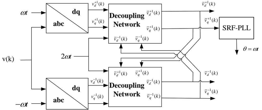
Figure 1.15: The control diagram of the DDSRF-PLL
