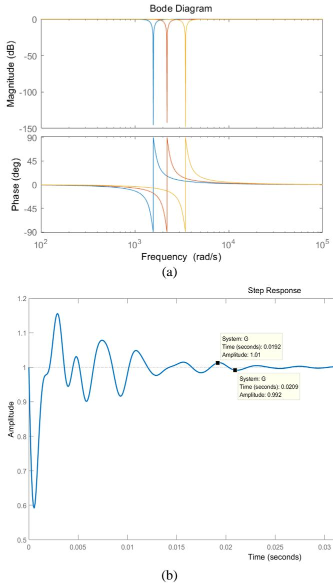
Figure 2.8: (a) The Bode diagram and (b) the step response of the notch filters
