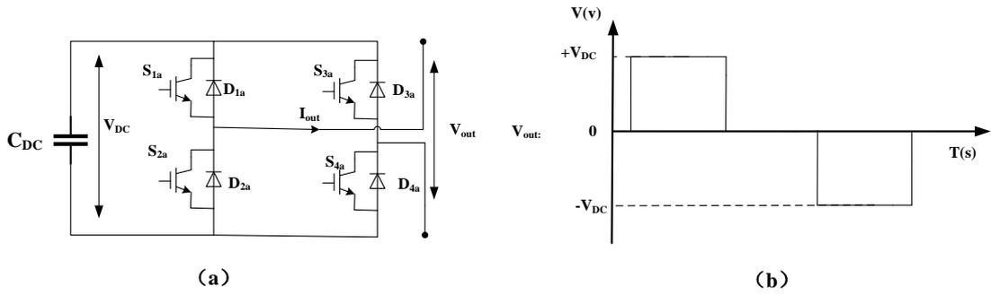
Figure 1.22: (a) Three-level single phase H bridge converter (HB) circuit (b) Voltage level
