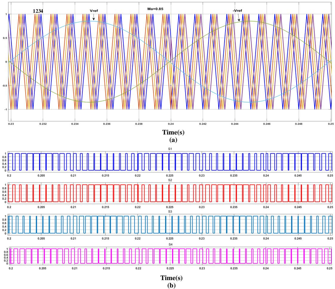
Figure 1.26: PS-PWM (a) Four carrier waves with the reference signals for nine-level CHB and (b) Pulse signals generated for the first sub-module
