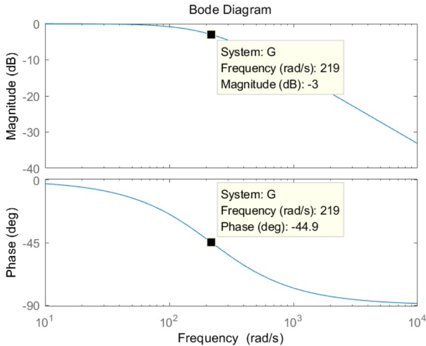
Figure 2.4: The Bode diagram of the low-pass filter when the cut-off frequency is 219.1 rad/s
