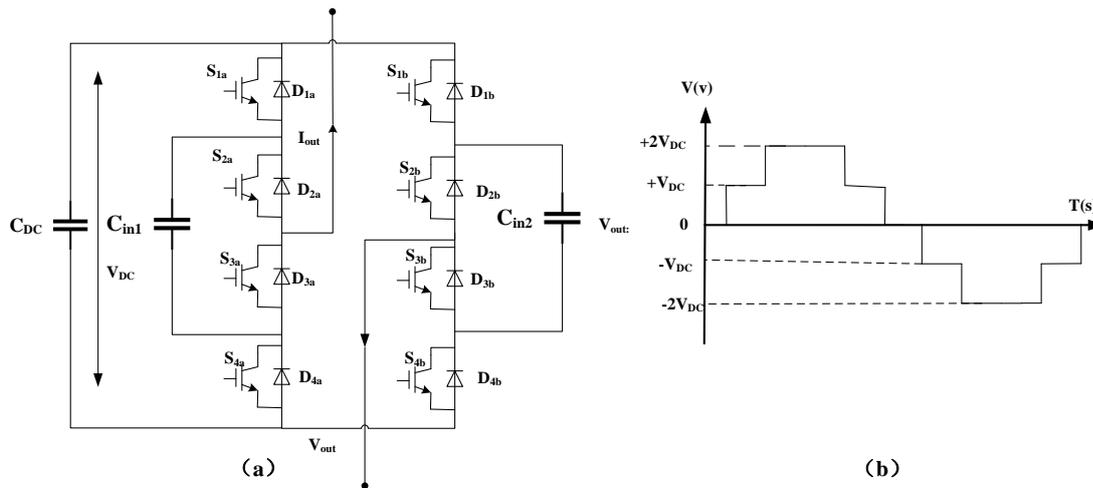
Figure 1.23: (a) Five-level Flying Capacitor Converter (FC) circuit (b) Voltage level
