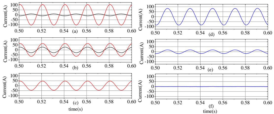
Figure 5.10: The circulating current (blue line) and the currents flowing into the SSSC1 branch (red line) and the SSSC2 branch (black line) (a) and (d) with the different reference current and without the circulating term in the cost function (b) and (e) with the different reference current and with the circulating term in cost function and (c) and (f) with same reference current and with the circulating term in the cost function.
