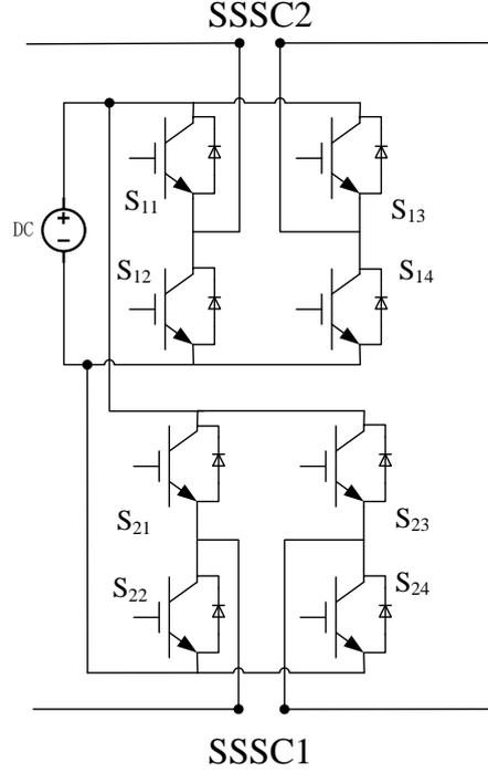
Figure 5.2: The single phase circuit diagram of a parallel TL-SSSC
