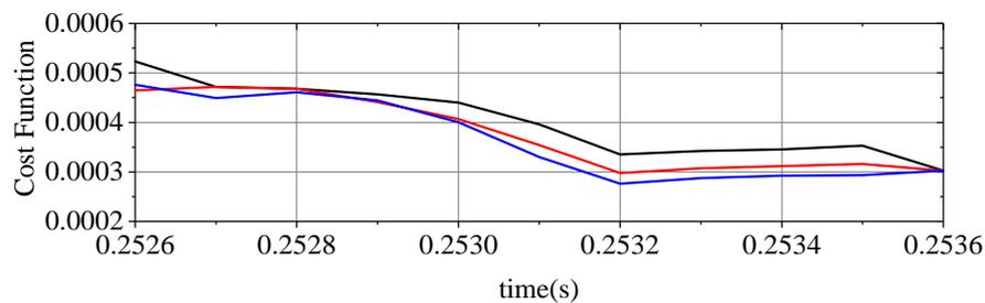
Figure 3.12: The cost function value comparison using different step size when the imbalance compensation ratio is 0.28.
