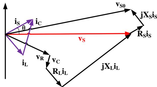
Figure 1.11: The phasor diagram of UPFC
