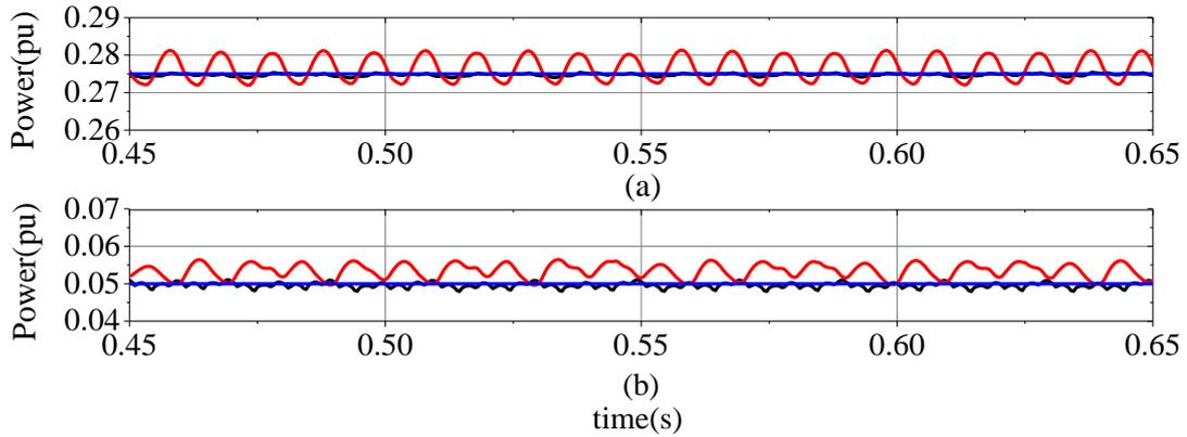
Figure 4.14: The receiving end measured powers compared to the reference powers (blue) (a) the active powers by the proposed method (black) and the conventional deadbeat method (red) (b) the reactive powers by the proposed method (black) and the conventional deadbeat method (red)
