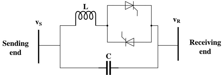
Figure 1.5: Thyristor Controlled series capacitor
