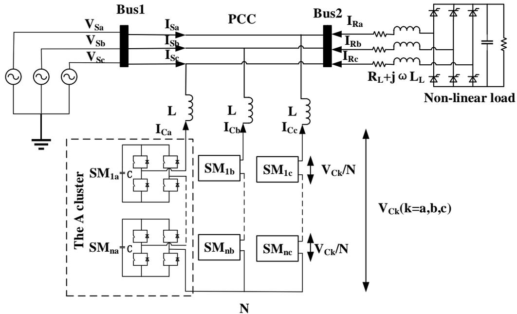
Figure 2.15: The configuration of MMCC-STATCOM.
