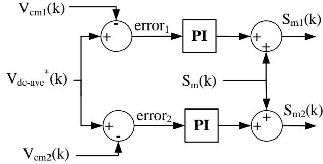
Figure 3.14: The diagram for the intra-cluster voltage balancing control block
