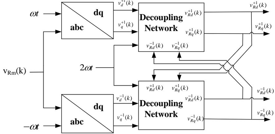
Figure 5.5: The schematic diagram of the DDSRF
