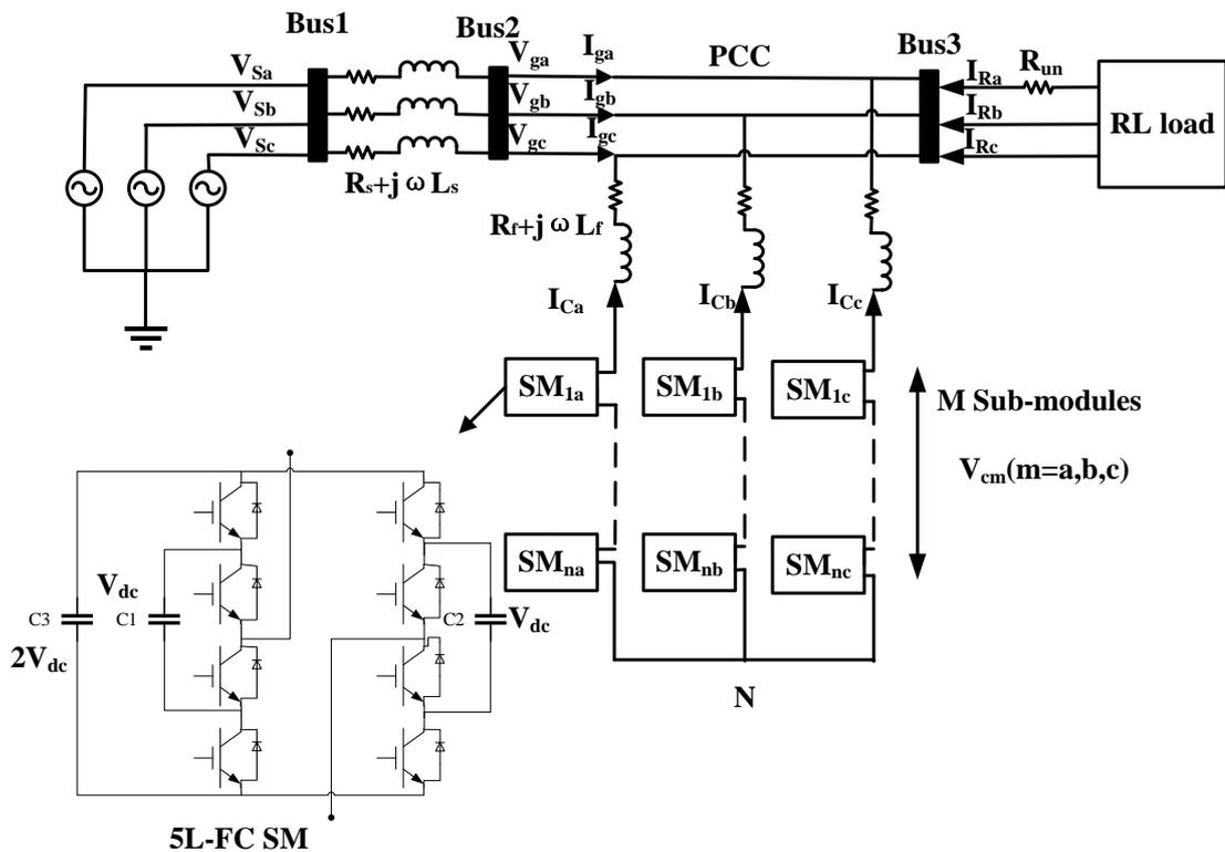
Figure 3.10: The configuration of a power system with the star-connected MMCC-STATCOM using the 5-level flying capacitor converter as sub-modules
