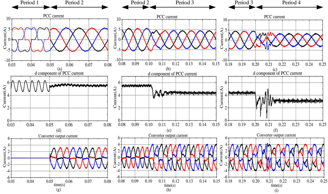
Figure 2.26: The variations of current waveforms using the method with data expansion:  $I_S$  (a) from period 1 to period 2 (b) from period 2 to period 3 (c) from period 3 to period 4.  $I_{Sd}$  (d) from period 1 to period 2 (e) from period 2 to period 3 (f) from period 3 to period 4. Compensation current  $I_C$  (g) from period 1 to period 2 (h) from period 2 to period 3 (i) from period 3 to period 4
