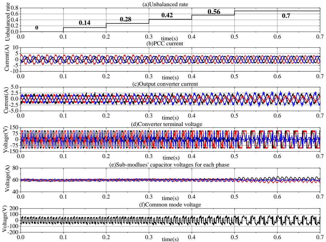
Figure 3.17: The experimental results (a) the Unbalanced rate (b) the PCC current (c) the output converter current (d) the converter terminal voltage (e) the sub-modules' capacitor voltages for each phase and (f) the common mode voltage for the proposed method when the  $\lambda= 0.49$
