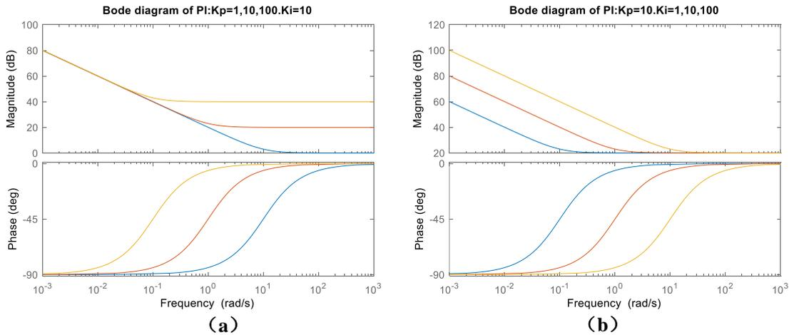
Figure 1.18: Bode diagram of PI controller (a) with different  $K_p$  and constant  $K_i$  (b) with different  $K_i$  and constant  $K_p$
