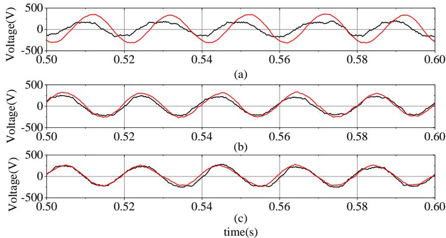
Figure 5.11: The measured phase A voltage for the SSSC1 (black line) and the SSSC2 (red line) (a) with the different reference current and without the circulating term in cost function (b) with the different reference current and with the circulating term in cost function and (c) with the same reference current and with the circulating term in the cost function
