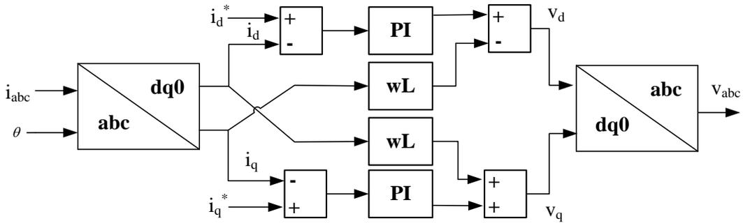
Figure 1.19: The current control diagram for a PI controller
