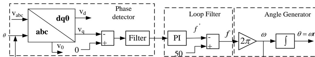
Figure 1.14: The control diagram of SRF-PLL with filter
