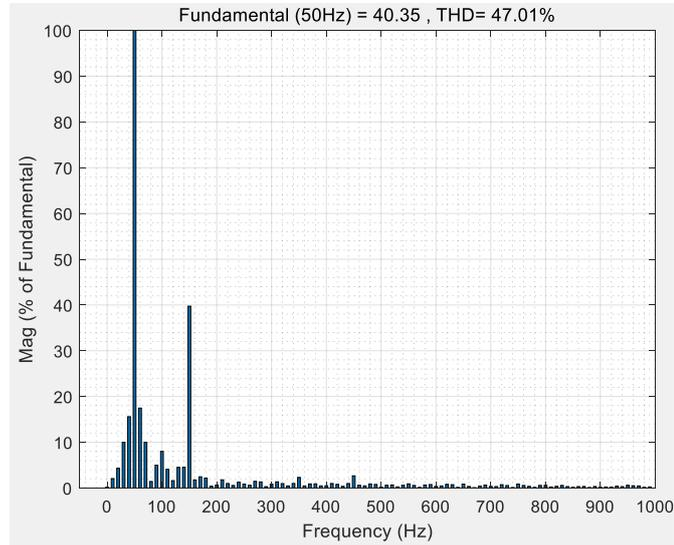
Figure 3.20: The frequency spectra of the common mode voltage when the unbalanced ratio is 0.42 for the conventional method
