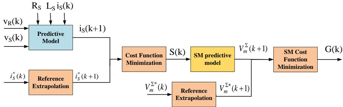
Figure 3.8: The control block diagram of the dual stages MPC
