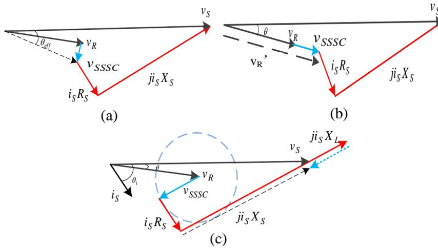
Figure 4.2: (a) The only active power control (b) the only reactive power control, (c) the line impedance control
