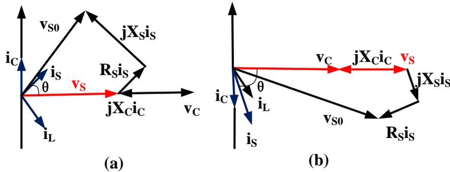
Figure 1.4: (a) Phasor diagrams when  $v_C > v_S$  (b) phasor diagrams when  $v_C < v_S$
