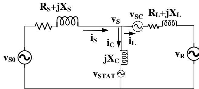
Figure 1.10: The equivalent circuit of Unified Power Flow Controller
