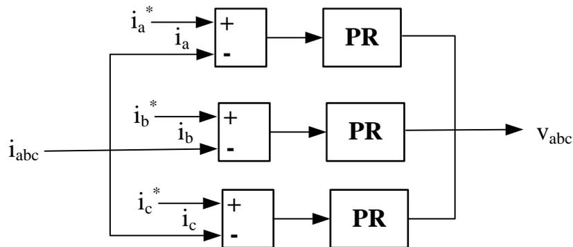
Figure 1.21: The current control diagram by PR controller
