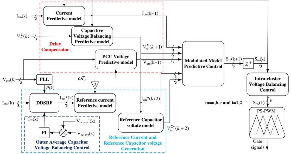
Figure 3.13: The overall control scheme of the MMPC for the MMCC-STATCOM
