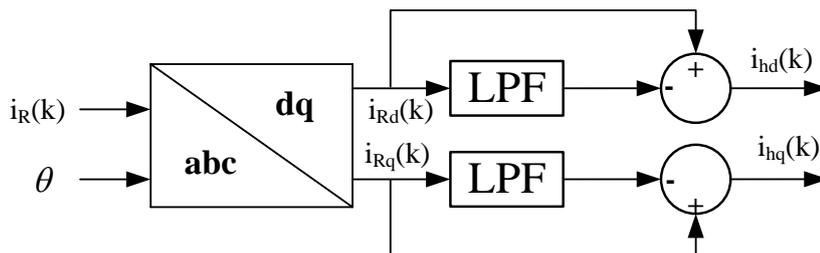
Figure 2.3: The Schematic diagram of the low-pass filter-based extraction method
