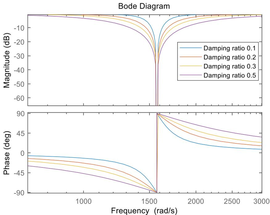
Figure 2.19: The bode diagram for the adaptive notch filters.
