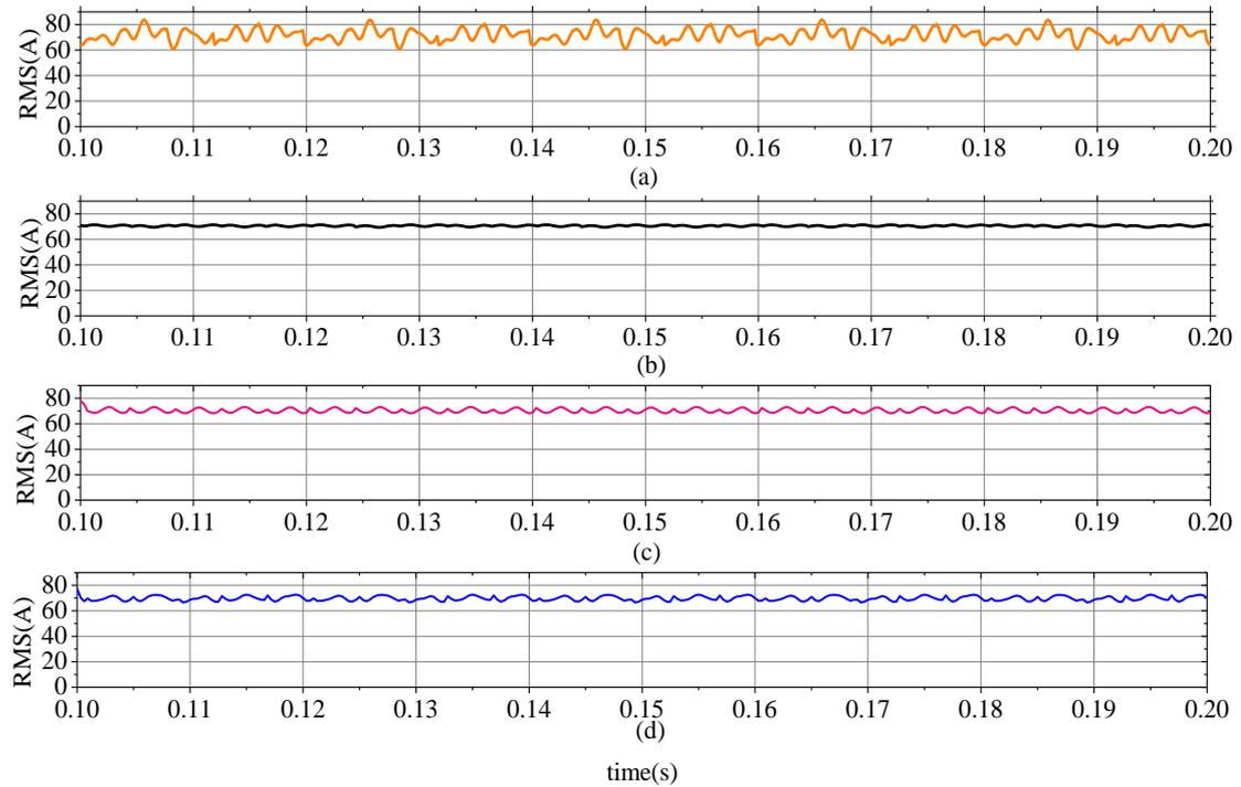
Figure 2.16: Reconstructed 5th order element by discrete meyer (a) without data expansion, (b) with data expansion expanding to 6400 samples (c)3200 samples and (d) 640 samples.
