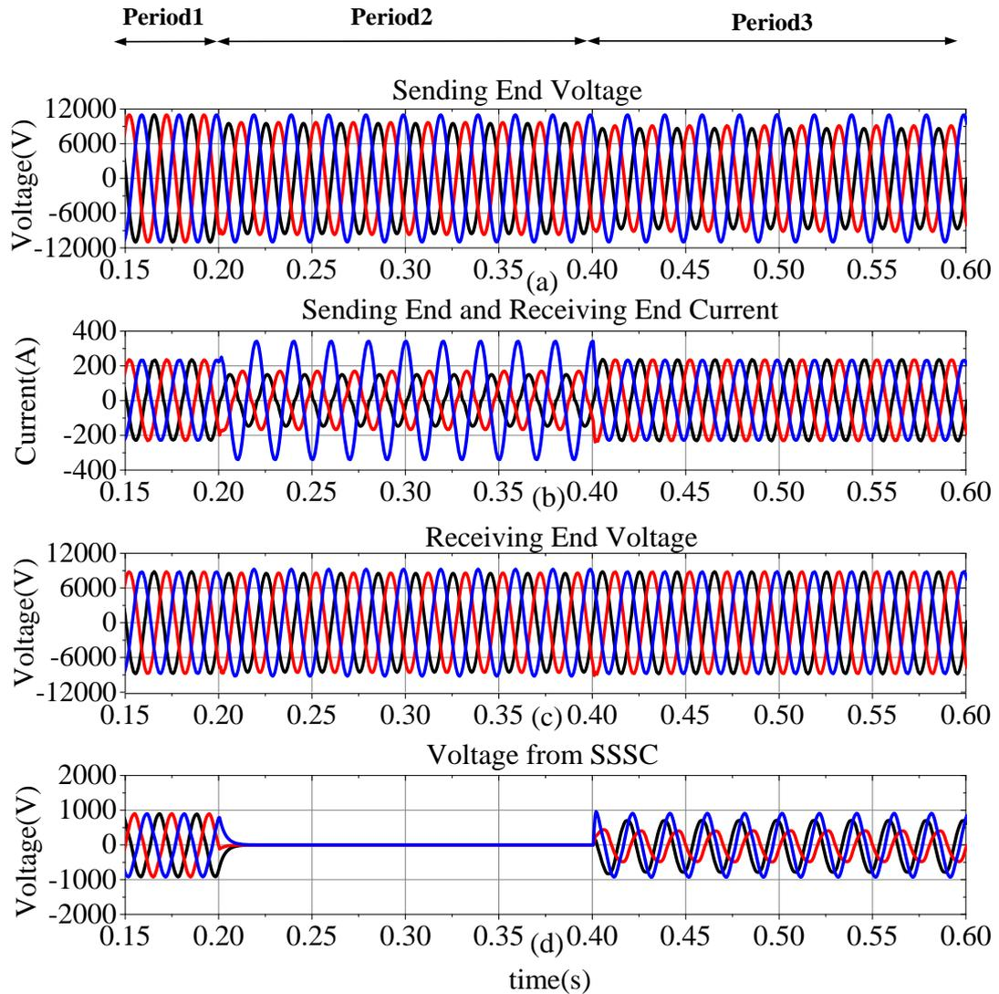
Figure 4.11: The measured waveforms from the proposed method for scenario 1 (a) the sending end voltages, (b) the sending end and receiving end currents (c) the receiving end voltages, (d) the TL-SSSC generated voltage for the double phase grounding fault
