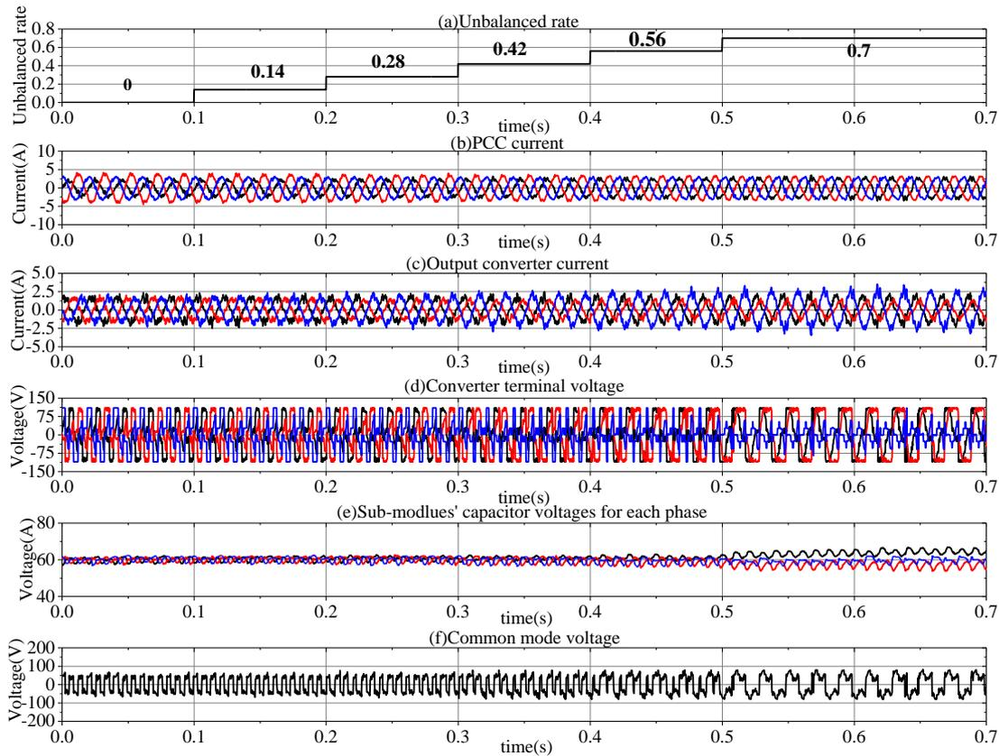
Figure 3.16: The experimental results (a) the Unbalanced rate (b) the PCC current (c) the output converter current (d) the converter terminal voltage (e) the sub-modules' capacitor voltages for each phase and (f) the common mode voltage for the proposed method when the  $\lambda = 0.25$
