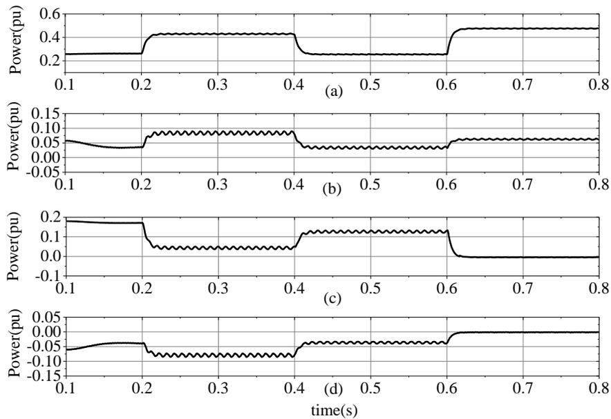
Figure 4.18: (a) The active power and (b) the reactive power at the receiving end (c) the active power and (d) the reactive power at inverters side over 4 periods
