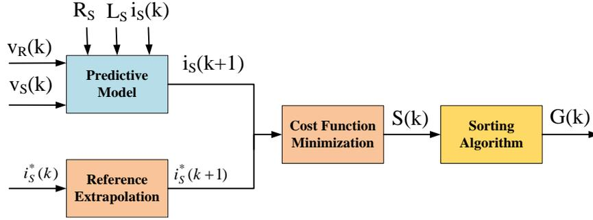
Figure 3.7: The control block diagram of the OVL-MPC
