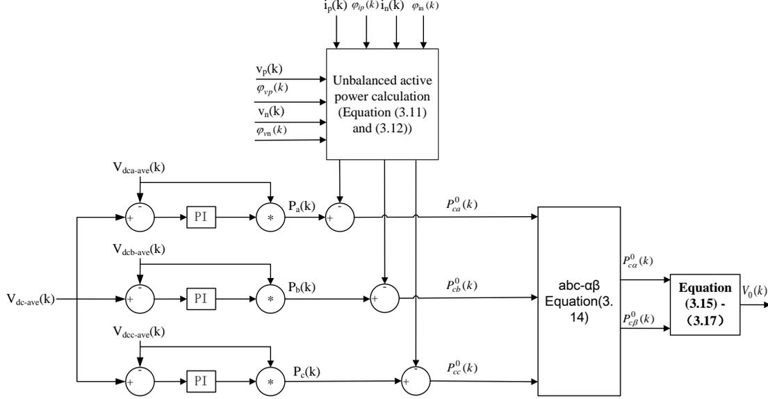
Figure 3.3: The block diagram for the zero sequence voltage calculation
