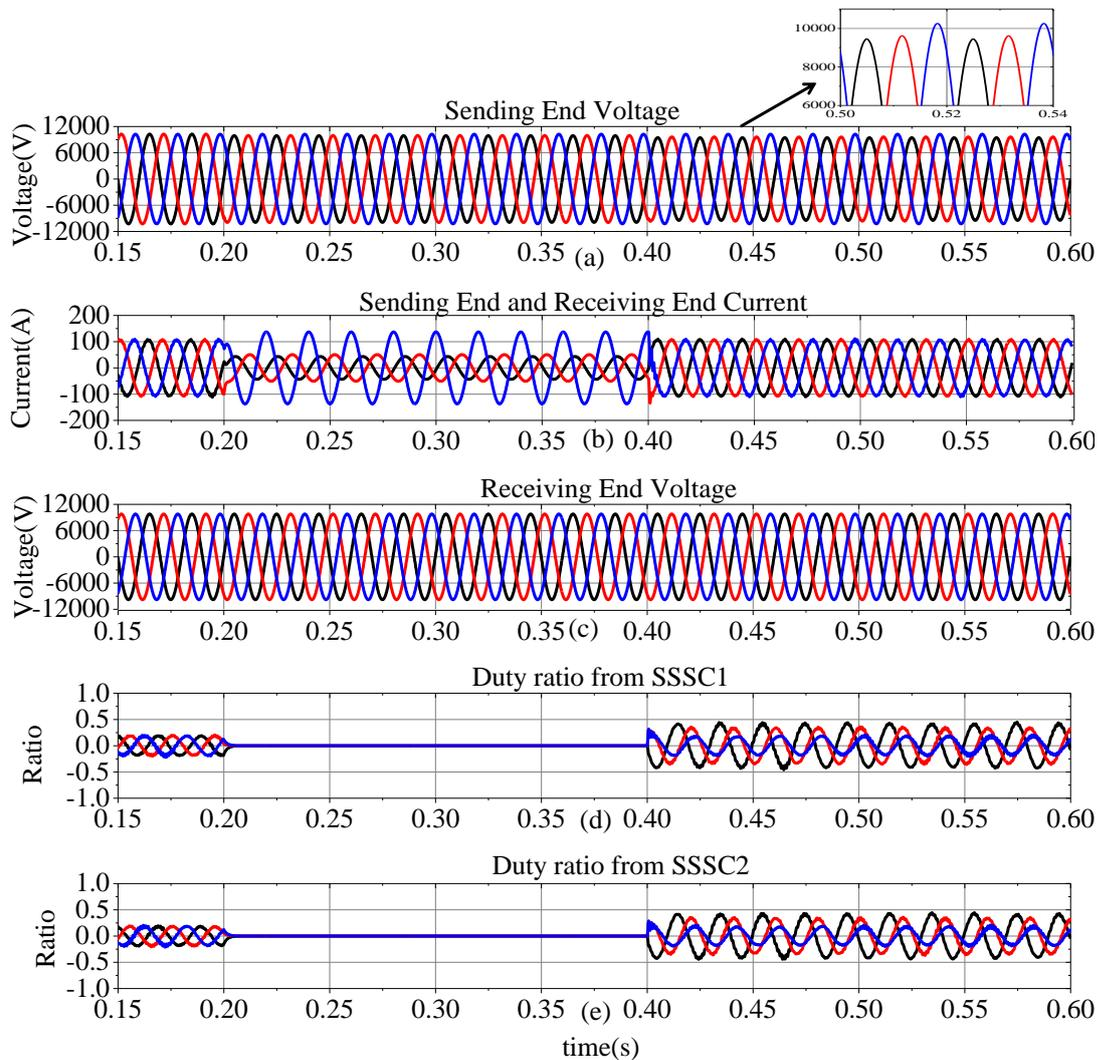
Figure 5.12: Scenario 1: the measured waveforms (a) the sending end voltages, (b) the sending end and receiving end currents, (c) the receiving end voltages, (d) the duty ratio for the SSSC1 and for (e) the SSSC2.
