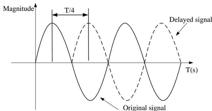
Figure 1.16: Demonstrating how the 2nd harmonic part is cancelled by DSC
