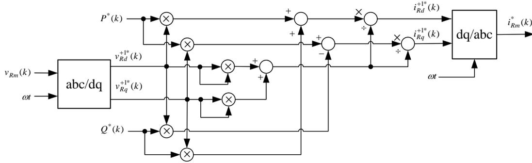
Figure 5.3: The diagram of the reference current generation for the balance case
