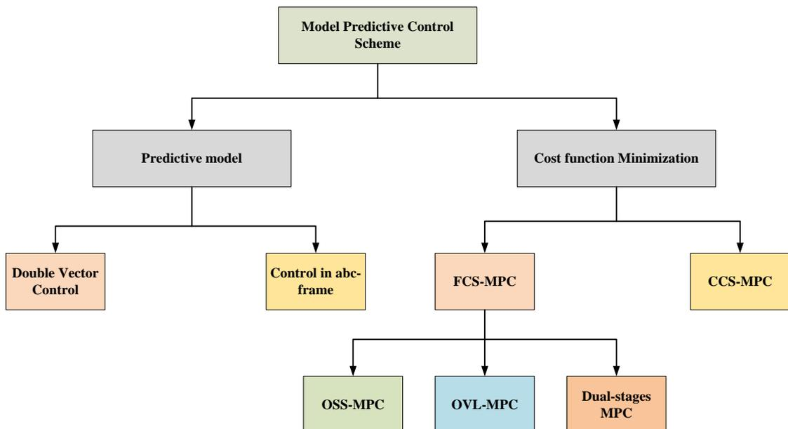
Figure 3.4: The different types of the MPC Control Schemes
