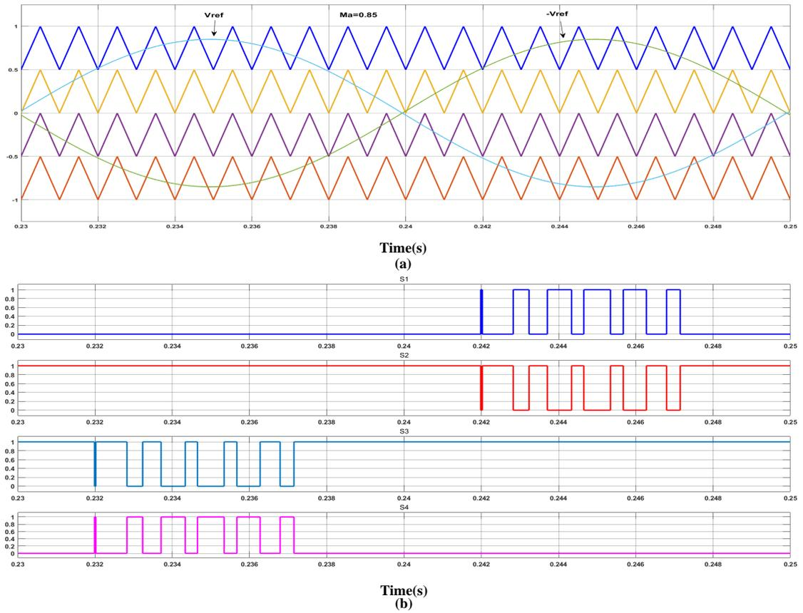
Figure 1.27: PD-PWM (a) Four carrier waves with the reference signals for nine-level CHB and (b) Pulse signals generated for the first sub-module
