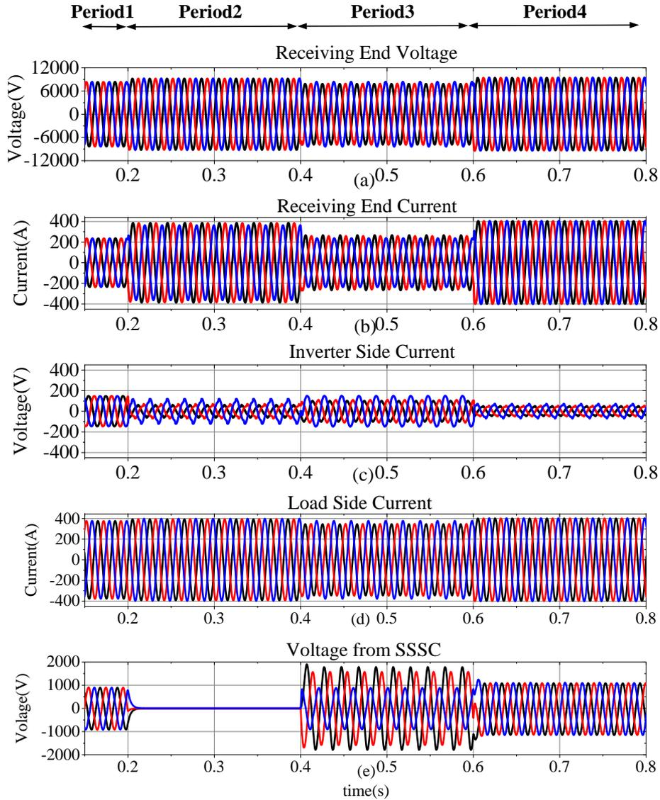
Figure 4.17: The measured waveforms from the proposed method for scenario 3 (a) the receiving end voltages, (b) the receiving end current (c) the inverter side current, (d) the load side current (e) the TL-SSSC generated voltage
