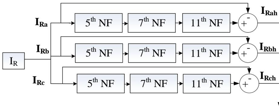
Figure 2.21: The implementation of a three-phase band pass filter.
