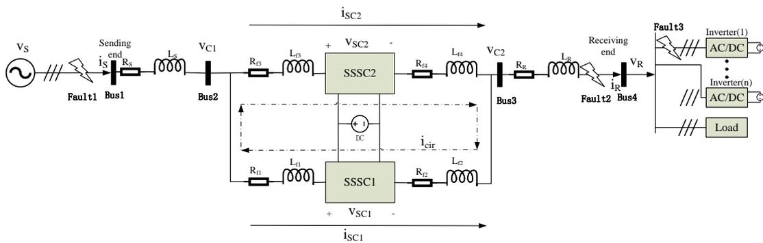
Figure 5.4: The configuration of a power line with a parallel TL-SSSC when the faults happen at different locations
