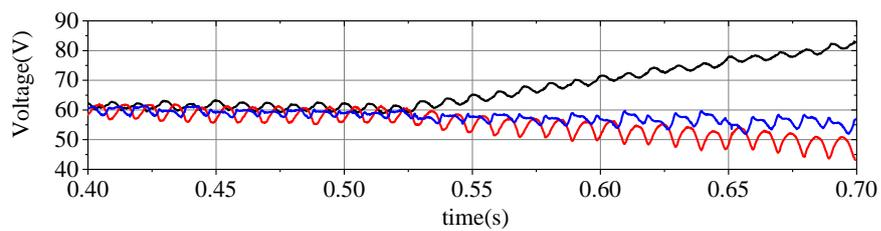
Figure 3.21: The variations of the sum of the sub-modules capacitor voltages with the  $\lambda=0.16$  and the compensation ratio 70%
