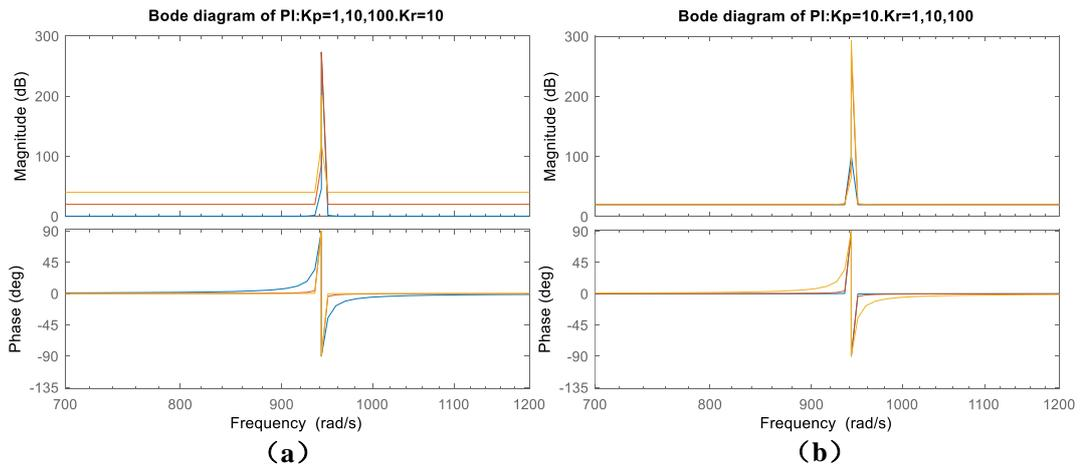
Figure 1.20: Bode diagram of PR controller (a)with different  $K_p$  and constant  $K_r$  (b) with different  $K_r$  and constant  $K_p$
