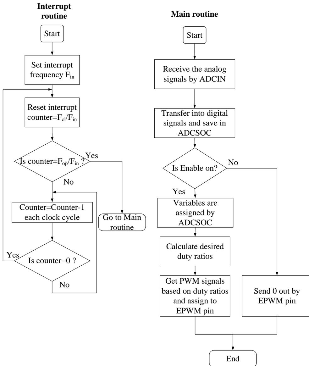
Figure 4.10: The flow chart of the operation stage for the DSP
