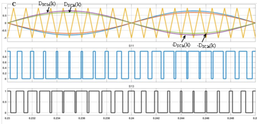
Figure 5.8: The uni-polar PWM for the parallel TL-SSSC and the PWM signals for the switches  $S_{11}$  for the SSSC1 and the  $S_{13}$  for the SSSC2
