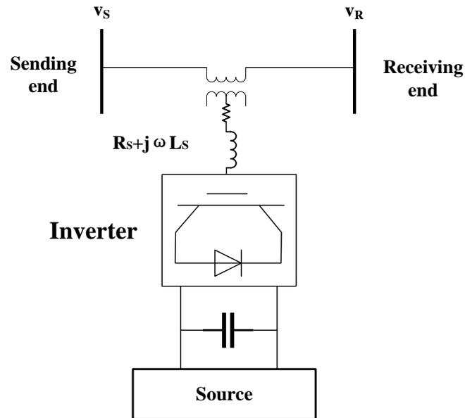
Figure 1.6: The configuration of Static synchronous series compensator
