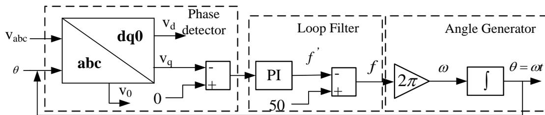
Figure 1.13: The control diagram of SRF-PLL
