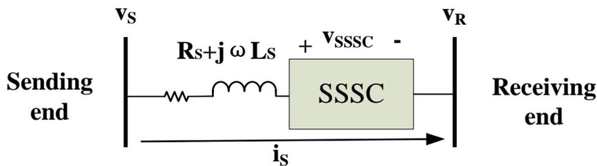
Figure 4.1: The power line with the SSSC
