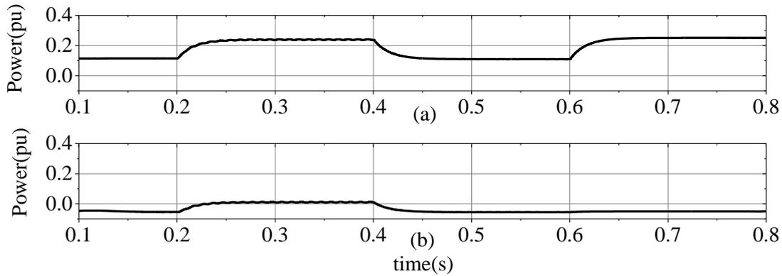
Figure 5.17: (a) The active power and (b) the reactive power at the receiving end
