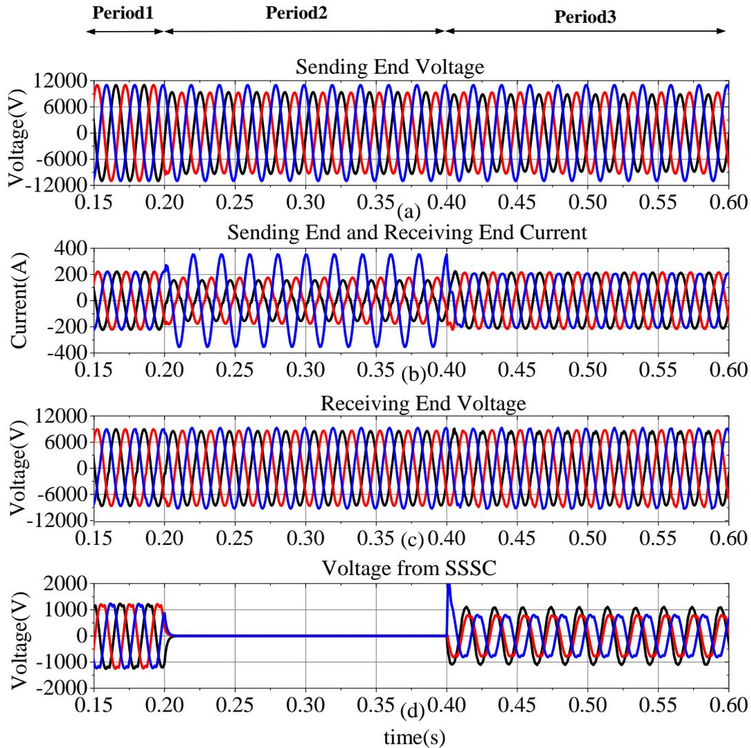
Figure 4.12: The measured waveforms from  $\pm$  sequence–based by Hilmy Awad method (a) the sending end voltages, (b) the sending end and the receiving end currents (c) the receiving end voltages, (d) the TL-SSSC generated voltage for the double phase grounding fault
