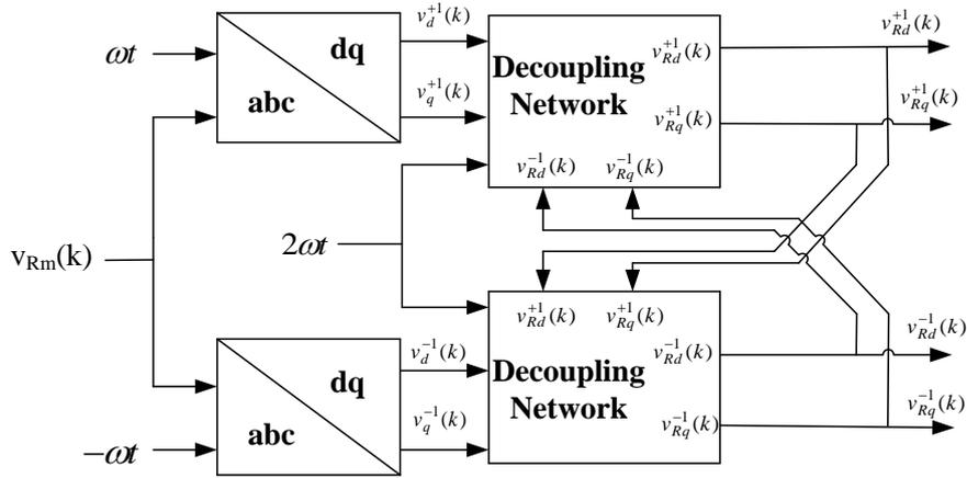
Figure 3.1: The schematic diagram of the DDSRF
