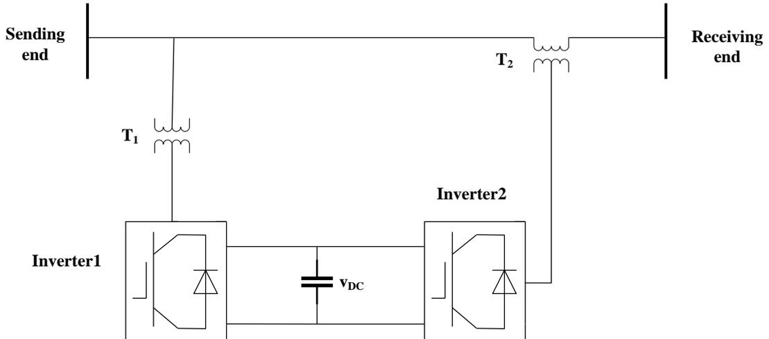
Figure 1.9: The configuration of Unified Power Flow Controller
