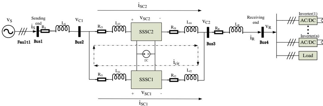
Figure 5.1: The configuration of a power line with a parallel TL-SSSC
