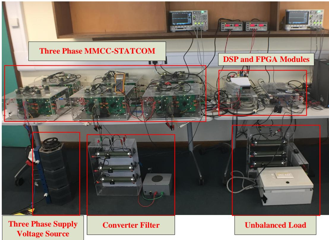
Figure 3.15: The MMCC-STATCOM prototype and the other system hardware components
