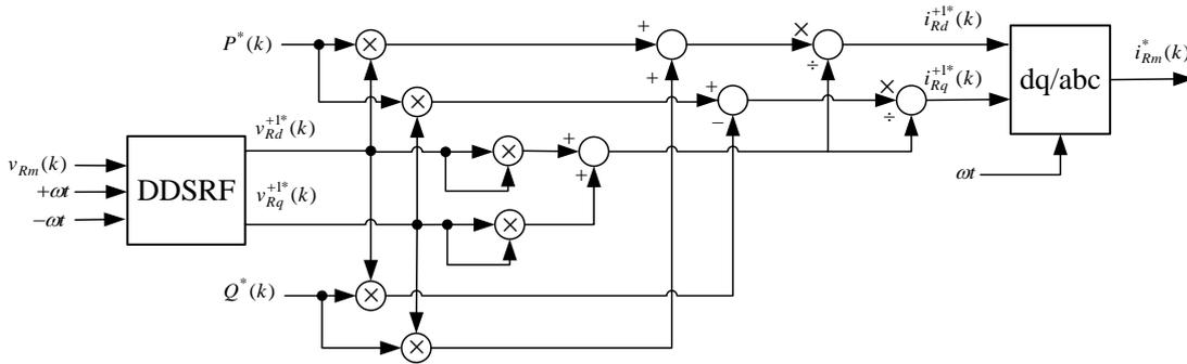
Figure 5.6: The block diagram for the reference current generation for the unbalanced voltage case
