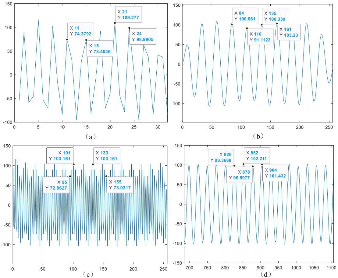
Figure 2.14: The reconstructed waveform by db30 wavelet function under (a) 800Hz and (b) 6400Hz for 0.04s and (c) 800Hz and (d) 6400Hz for 0.32s
