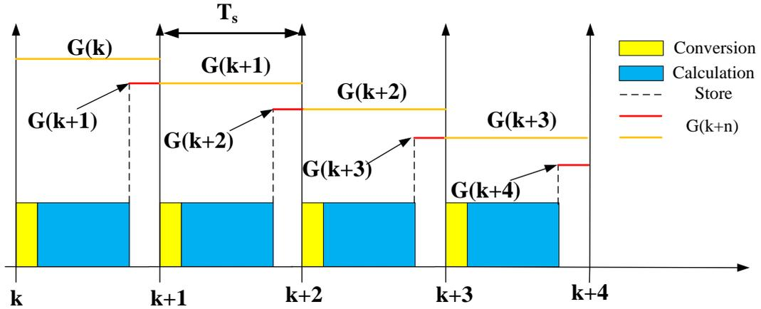
Figure 4.4: The time diagram for the digital control system
