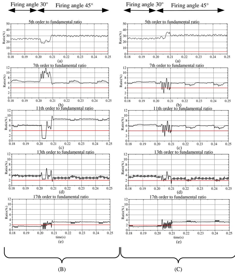
Figure 2.24: The variations of the 5th, 7th , 11th, 13th and 17th harmonic to fundamental ratio identified by the DWPT with the data expansion. B When the power system frequency is 49.5Hz and the firing angle is from 30° to 45°: (a) 5th order (b) 7th order (c) 11th order (d) 13th order (e) 17th harmonic. C When the frequency is 50.5Hz and the firing angle is from 30° to 45°: (a) 5th order (b) 7th order (c) 11th order (d) 13th order (e) 17th harmonic
