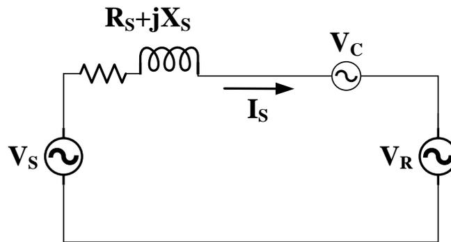
Figure 1.7: The equivalent circuit of Static synchronous series compensator
