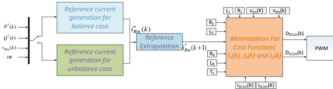
Figure 5.7: The overall control diagram of the parallel TL-SSSC
