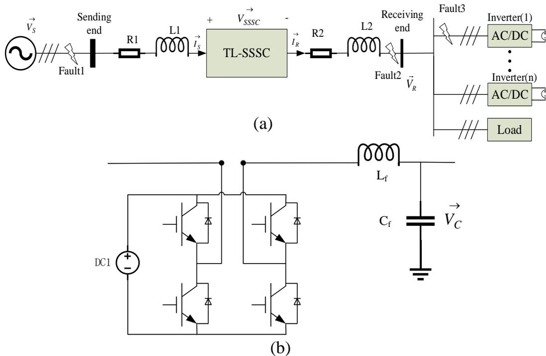
Figure 4.3: (a) The configuration of a power line with a TL-SSSC (b) the converter circuit configuration and the filter for each phase of a TL-SSSC
