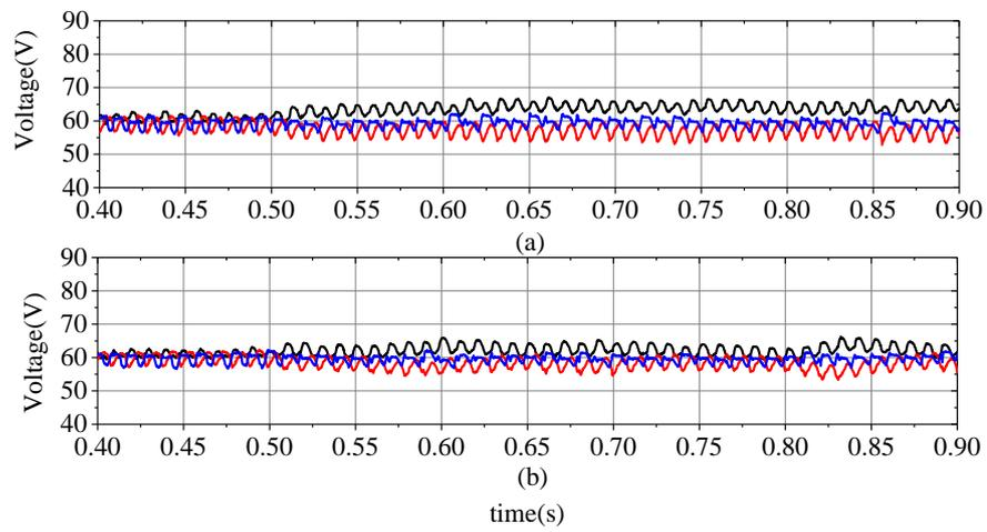
Figure 3.22: The variations of the sum of sub-modules capacitor voltages with (a) the  $\lambda=0.25$  and (b) the  $\lambda=0.49$  when the compensation ratio is 70%
