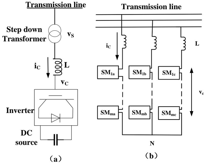
Figure 1.2: Static synchronous compensator (a)conventional STATCOM (b)MMCC-STATCOM
