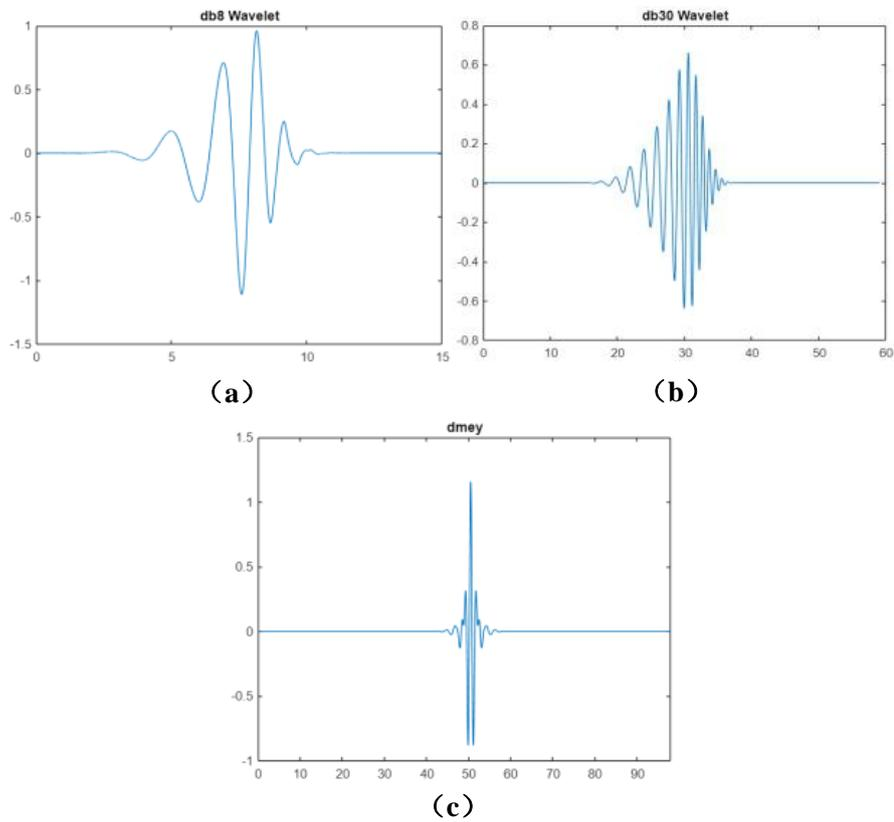
Figure 2.12: The mother wavelet function (a) db8, (b) db30 and (c) discrete meyer
