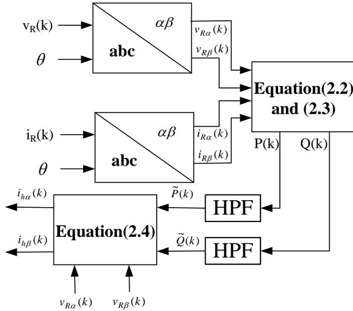
Figure 2.7: The control diagram of the high-pass filter-based extraction method
