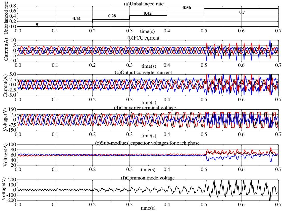
Figure 3.18: The experimental results (a) the unbalanced rate (b) the PCC current (c) the output converter current (d) the converter terminal voltage (e) the sub-modules' capacitor voltages for each phase and (f) the common mode voltage for the conventional zero sequence voltage injection method
