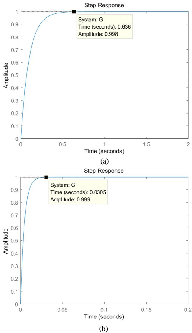
Figure 2.5: (a) The step response of the low-pass filter when the cut-off frequency is 10 rad/s (b) the step response of the low-pass filter when the cut-off frequency is 219.1 rad/s
