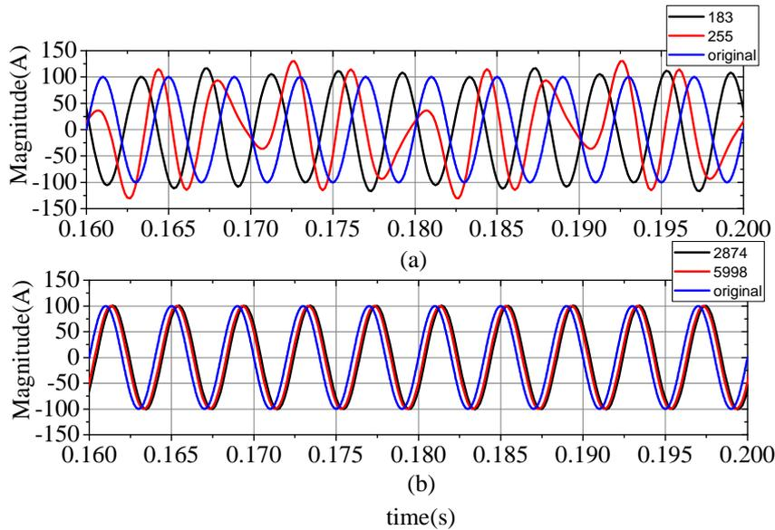
Figure 2.17: Reconstructed signals by choosing different points (a) without and (b) with data expansion.
