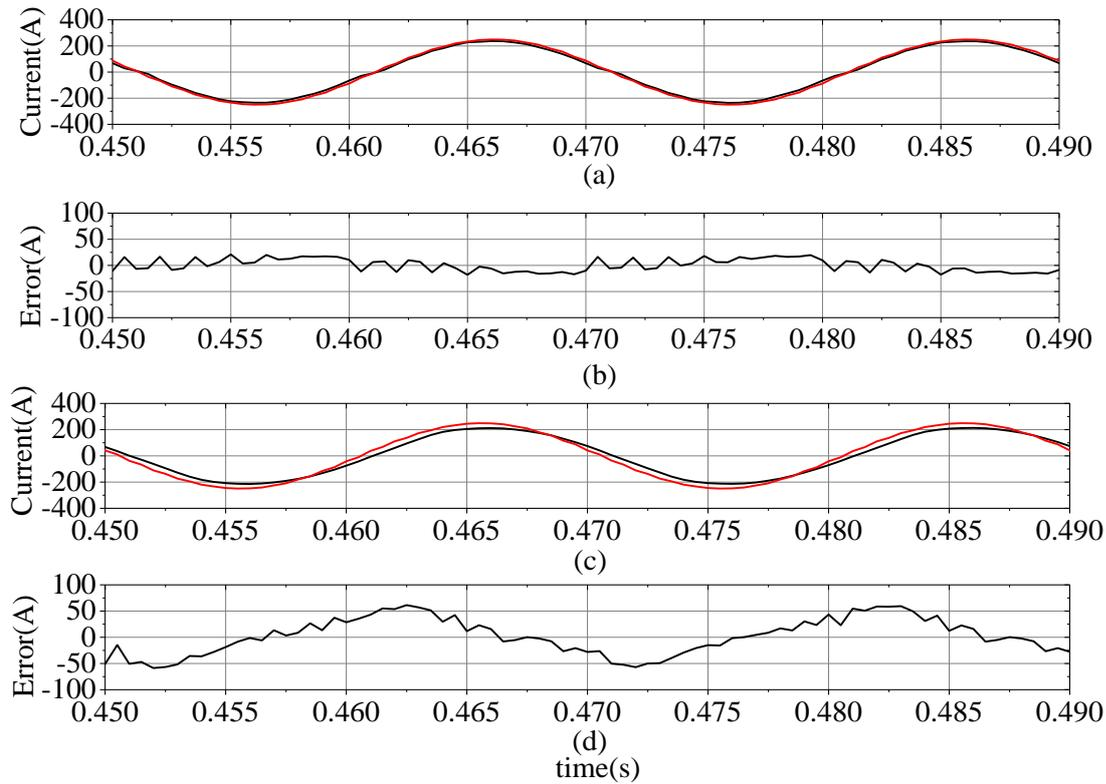
Figure 4.13: The receiving end (a) the waveform of reference (red) and the measured (black) current for the proposed method and (b) the error between these two waveforms (c) the waveform of the reference (red) and the measured (black) current for the conventional method and (d) the error between these two waveforms
