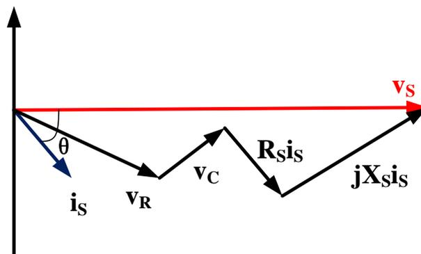
Figure 1.8: The phasor diagram of SSSC
