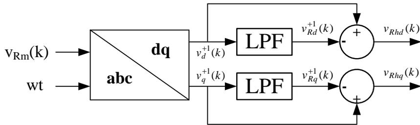
Figure 3.2: The schematic diagram of the low-pass filter method
