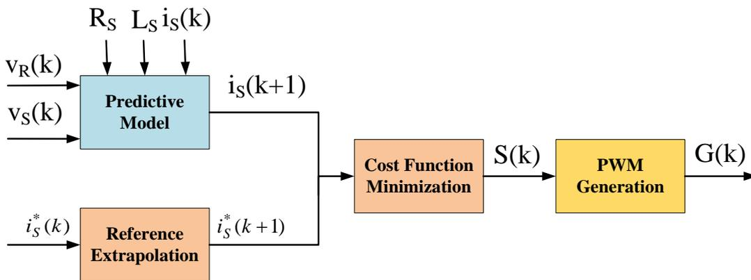
Figure 3.9: The control block diagram of the CCS-MPC
