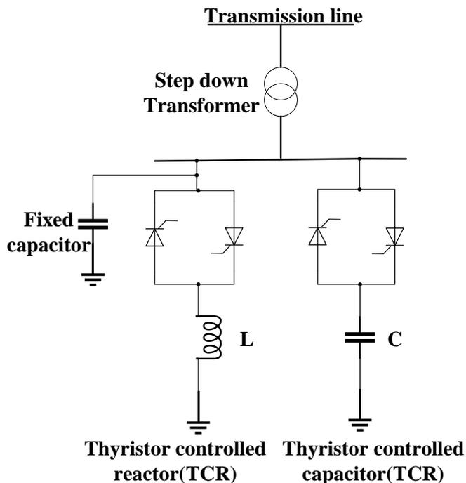
Figure 1.1: Static VAR Compensator
