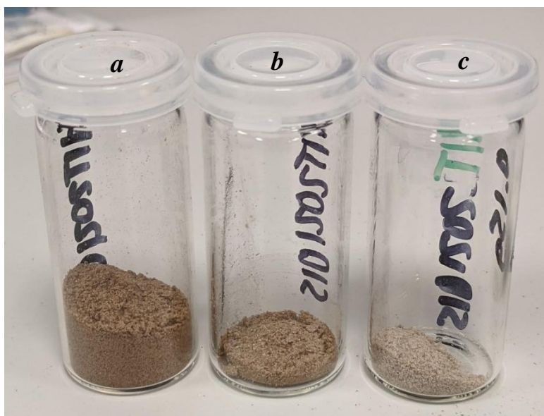
Figure 91: Photographic images of the products resulting from BSFL chitin and chitosan extraction, where pigment loss can be seen at each stage ( a : BSFL demineralisation product, b : BSFL chitin and c : BSFL chitosan)
