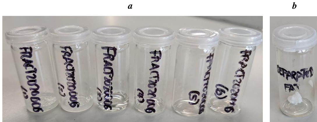
Figure 29: BSFL oil distillation of resulted in colourless oil following distillation (a) of FAMES and (b) FFAs after reverse esterification
