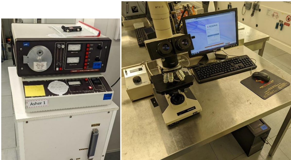
Figure 3.12: a) The resist asher. b) Microscope system to view samples
