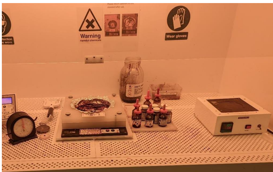
Figure 3.1: Photoresist control unit on a chemical bench with resist phials, a timer, and a hotplate.
