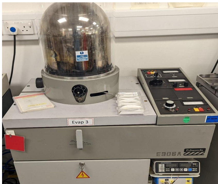
Figure 3.10: An Edwards E306A Thermal Evaporator and its bell jar, with a crystal monitor. A separate cylindrical implosion jar is also used.
