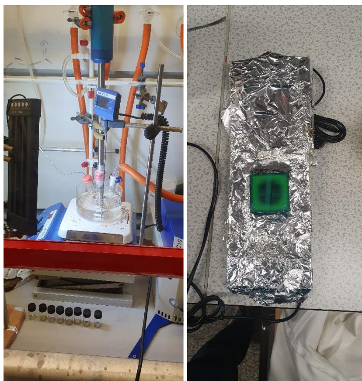
Figure 229. Left: LED array set up for reaction. Right: Foiled LED Array for controlled wavelength experiments.
