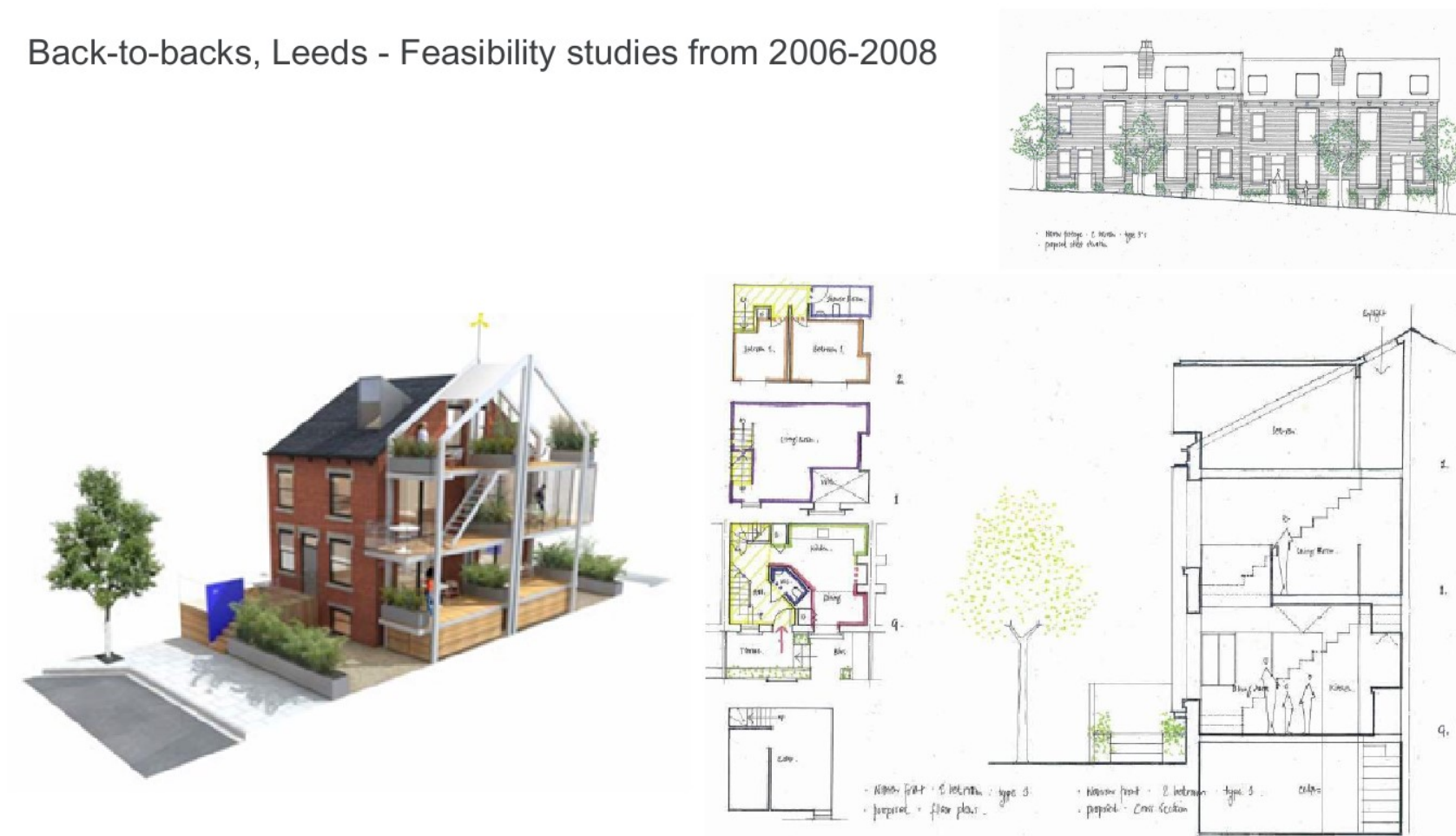
Figure 119 Workshop 2 Task 1, Aspirations: Appraisal of Back-to-backs, Leeds. This feasibility study for Leeds explored the potential of reconfiguring the houses individually, as well as combining them sideways and 'front to back.' The appearance of the houses was modernised and a contemporary intervention in the bin yard spaces showed multi-level outdoor amenity space (Images: Barraclough, Horner and Jones 2008b, 56-57; LCC 2006a, 12).
