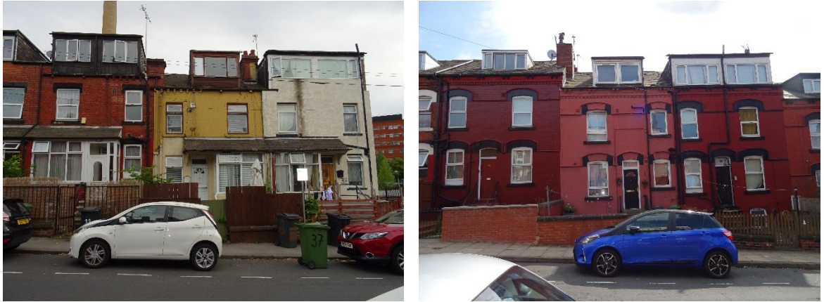
Figure 26 The massing and construction material of dormer windows has eroded the uniformity of the streetscape which was a significant element of the neighbourhood's original design and character (Harrison 2019).
