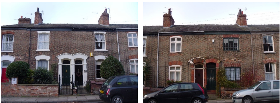
Figure 64 Although many of the houses in the Bishophill area of York retain much of their original fabric (left), there are still examples of attempts to individualise properties, such as changes to the fenestration (right).
