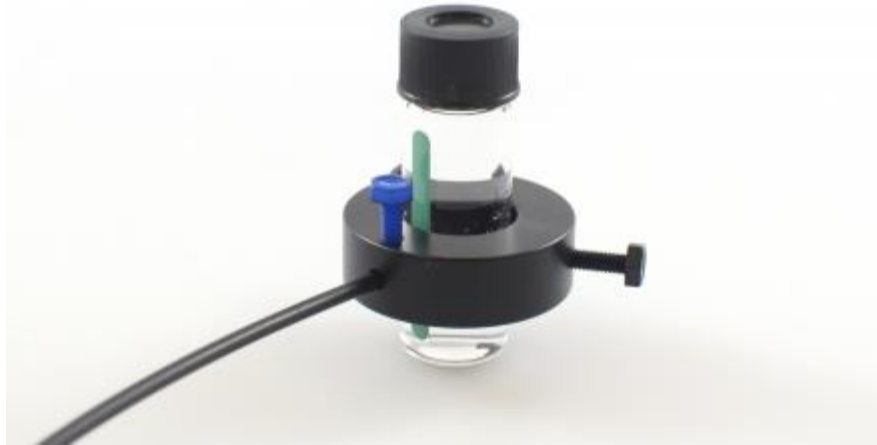
Figure 3.4: closed circuit respirometry vial as used to measure change in dissolved oxygen
