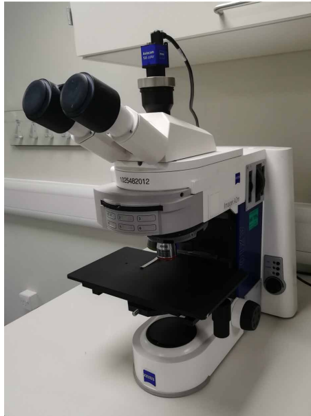
Figure 3.2: Zeiss AX10 optical microscope used for detailed surface damage observation.
