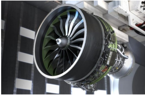
Figure 1.1. Photos of two sophisticated engineering examples demanding the highest possible reliability. (a): General Electric GE9x: World's most powerful commercial aircraft jet engine delivering 134,300 lbs of thrust. Photo from [6]. (b): Akashi Kaikyo: World's largest suspension bridge, designed to resist typhoons of 180 mph and earthquakes up to 8.5 on the Richter scale. Photo from [15].
