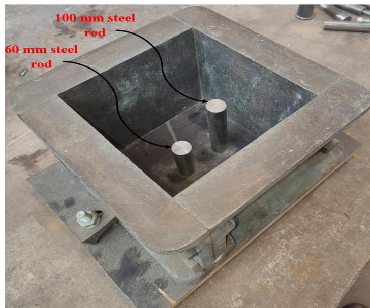
Figure 2.3 Steel mould with preinstalled steel rods.
