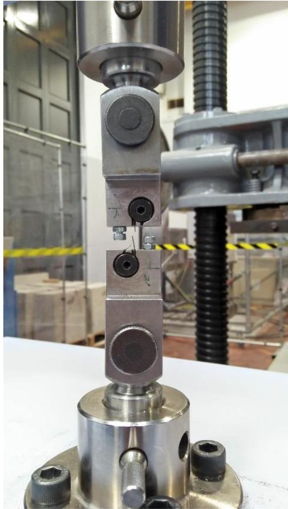
Figure B.1 Tensile test setup.
