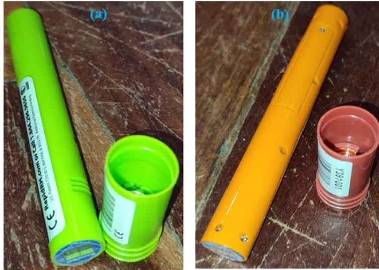
Figure 2.1 Humidity Sensors; (a) Rapid RH L6, (b) Rapid RH 5.0.
