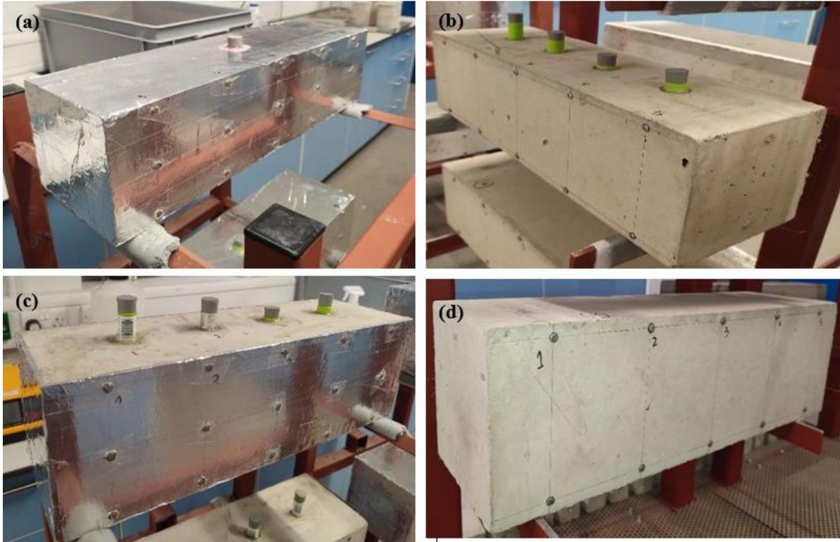
Figure 4.3 Instrumented test specimens: (a) CS with one RH sensor; (b) ASE with four RH sensors; (c) OSE with four RH sensors; (d) ASE without sensors
