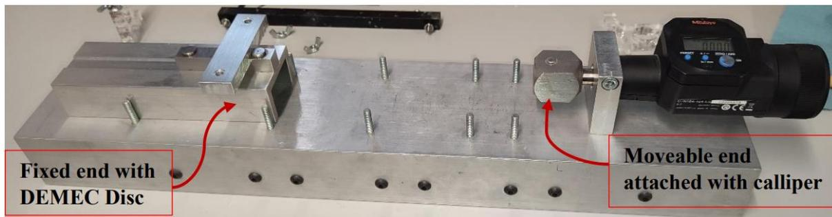
Figure 2.16 Calibration rig.
