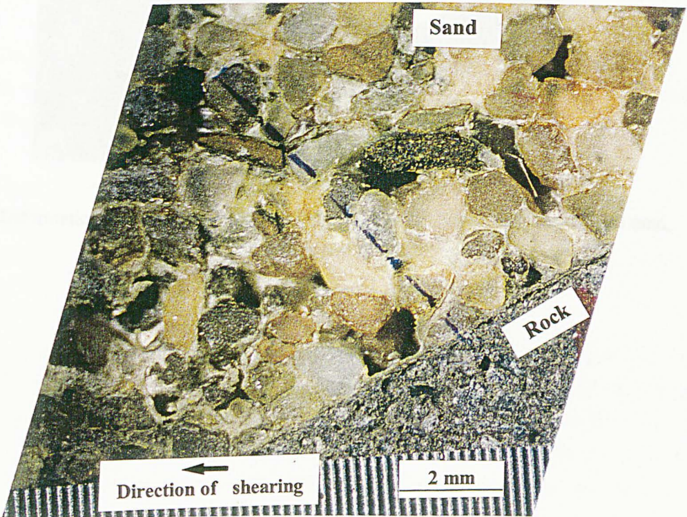
Plate 8.3: Load bearing bridges formed when a sand is sheared on top of a rock saw-toothed surface under a normal stress of 400 kPa
