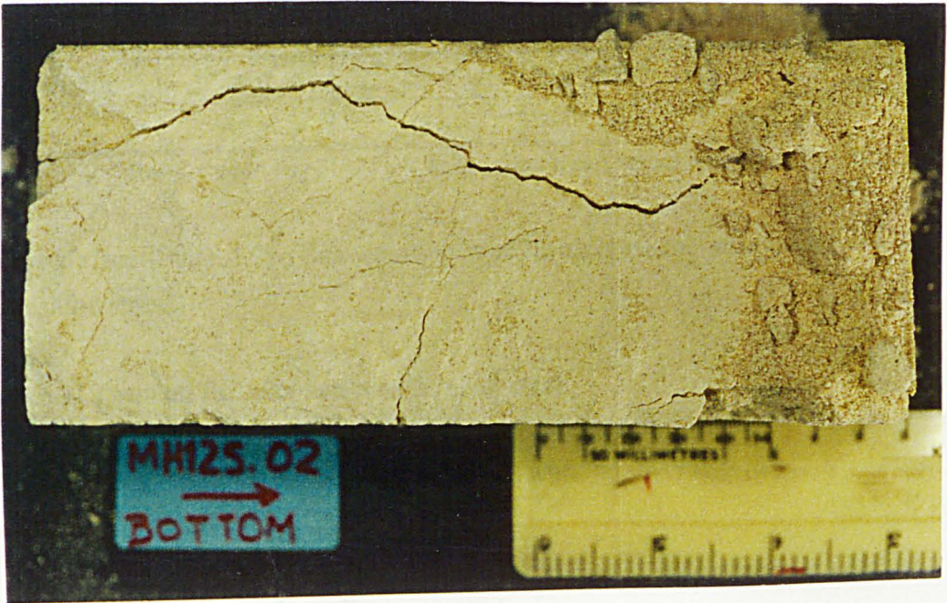
Plate 4.6: Deformation of medium-sized block under a normal stress of 125 kPa
