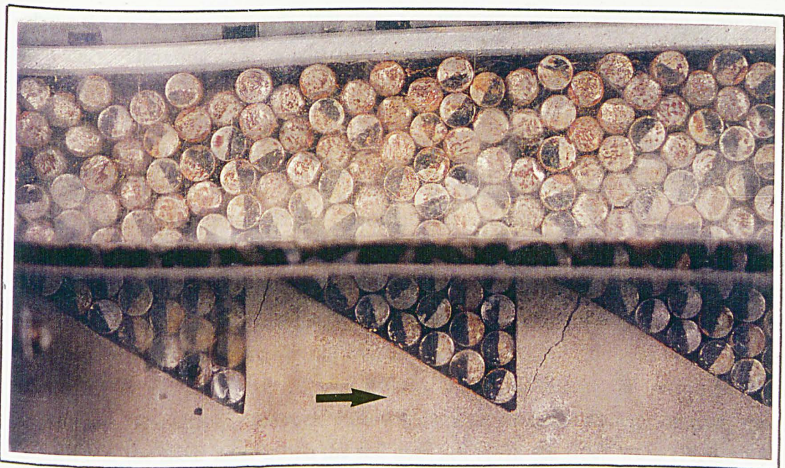
Plate 8.2: Tensile failure of teeth of a rock saw-toothed surface sheared with an assembly of 3 mm steel rods under a normal stress of 400 kPa
