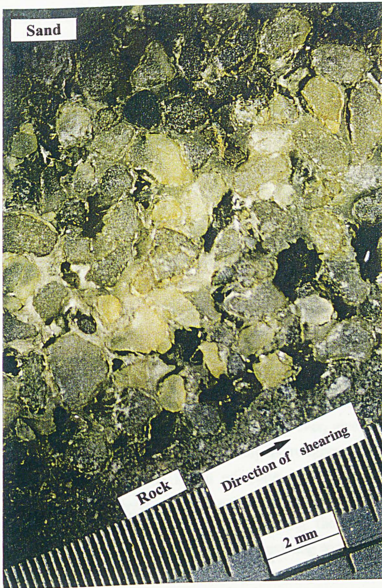
Plate 8.4: Deformation near a single interface between a rough planar rock surface and sand, tested under a normal stress of 400 kPa.
