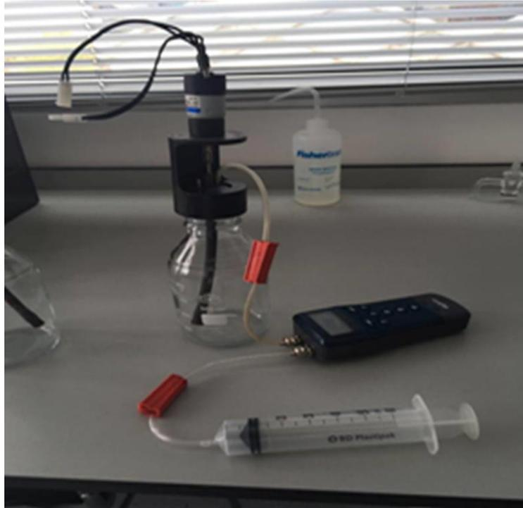
**Figure 3.2 Leak testing of batch reactor**
