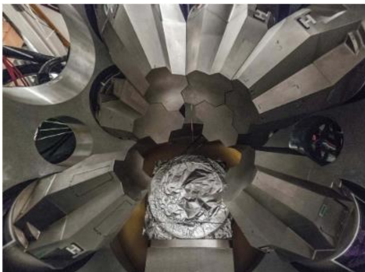
Figure 3.4: The positions of 7 HPGe modules applied in GRETINA from Ref. [86] being directed at the secondary 188 \text{ mg/cm}^2 target that is placed within the six-inch diameter beam line. Four of these modules are centered at 58^\circ with respect to the beam axis and the remaining three of these modules are centered around 90^\circ .
