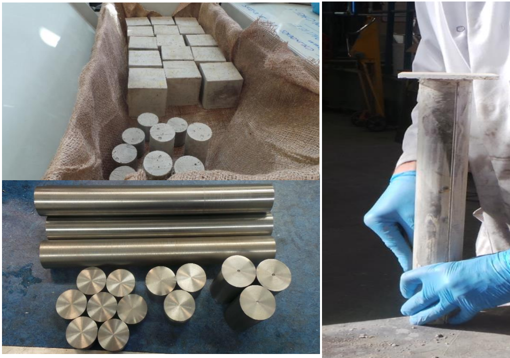
Figure 3.2 photos show steel strikers and samples as well as casting process of concrete in laboratory
