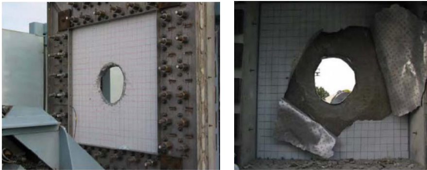
Figure 2.10 Experiments on the impact of aircraft to concrete panel (Sadiq et al., 2014)
