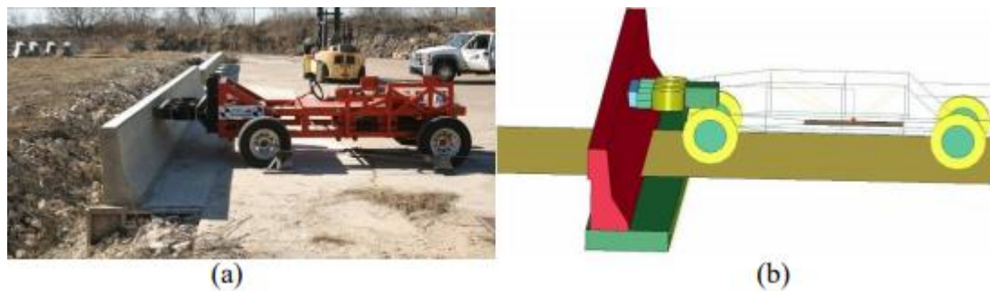
Figure 2.14 Experimental work on the impact of bogie against the concrete barrier (b) numerical simulation of bogie test in LS-DYNA (Abu-Odeh, 2015)
