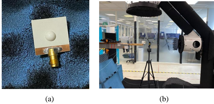
Figure 3.16: Photographs of (a) Hemispherical DRA with added substrate (b) Hemispherical DRA in the anechoic chamber.
