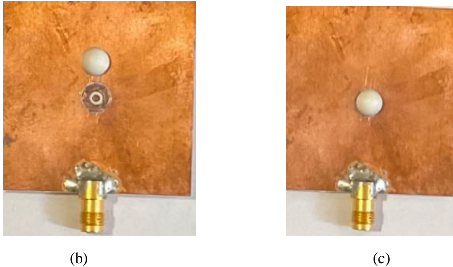
Figure 2.13: A hemispherical DRA above a grooved ground plane; (a) 3-D layout, (b) Fabricated grooved ground plane, (c) Assembled DRA.
