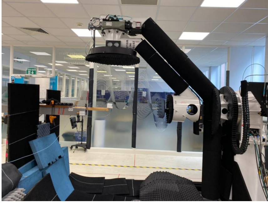
Figure 4.13: The prototype of rectangular DRA inside the anechoic chamber.
