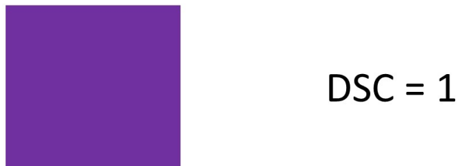
Figure 2.12: The Dice Similarity Coefficient is used for evaluating agreement between segmentations. It is based on the ratio between overlapped area to the total area of the two compared segmentations with one being a perfect agreement and zero being no overlap.
