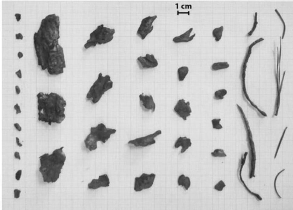
*Figure 2.3. The firebrand samples were collected in a prescribed fire conducted in a pine forest [20]. The variety of the shape and size indicate that in real wildland fire, the firebrand's shape is complicated. However, most of them are shown as a plat that has a relatively large cross-section area with a little thickness. Therefore, in the investigation of this thesis, the shape of the firebrand is simplified as a rectangular plate.*
