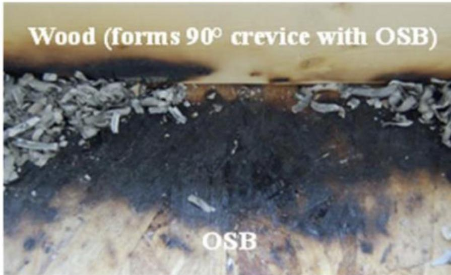
*Figure 2.21. The generated firebrand landing around the obstacle[50].*
