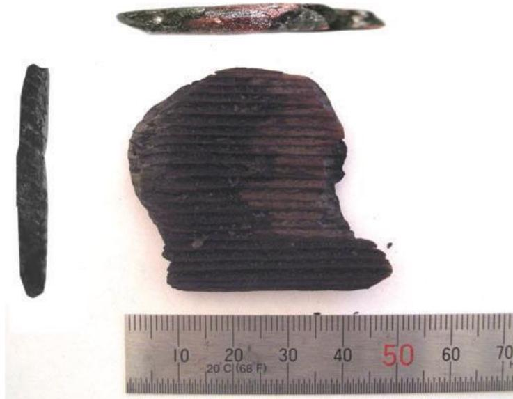
*Figure 2.2. A real firebrand from Oakland Wildfire. About 50mm in diameter, 5mm in thickness, and 2.3g in weight [40]. As it had burnt during transportation, the initial size of it should be larger. And this dimensional information of the firebrand will be utilized in the following mathematical modelling. And in the comparison of the experimental study of the firebrand.*
