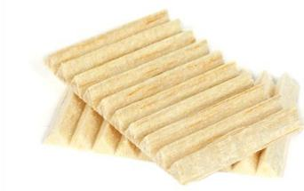
*Figure 3.1. The wooden smoke filter that being chosen as the sample of the firebrand.*
