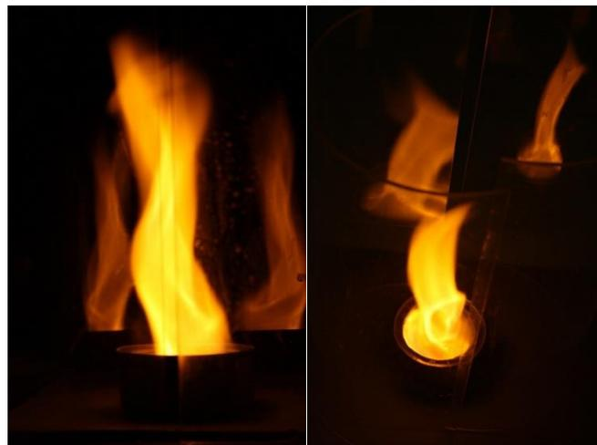
*Figure 3.5. The fire whirl is generated by a 98% volume fraction of liquid alcohol in the pool, of which the diameter is 50 mm.*
