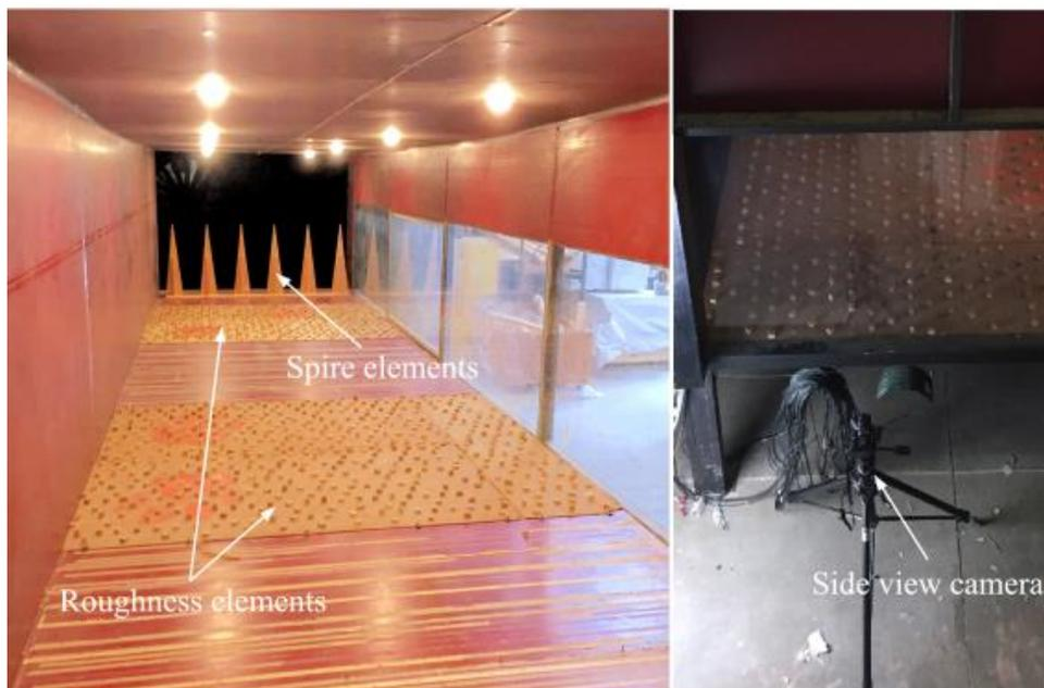
*Figure 2.15. Two side views about the setup of Ali Tohidi's experiment [80]. In the left-hand figure, in the horizontal wind tunnel, the roughness elements and spire elements have been introduced to generate a turbulence boundary layer. In the right-hand figure, a side view camera has been utilized to track the trajectory of firebrands.*
