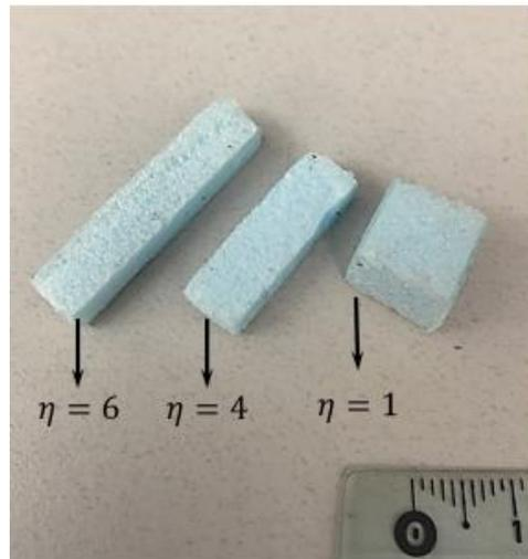
Figure 2.18. the polyurethane-made sample of a firebrand, with the aspect ratio  $\mu=1,4,6$  [80].
