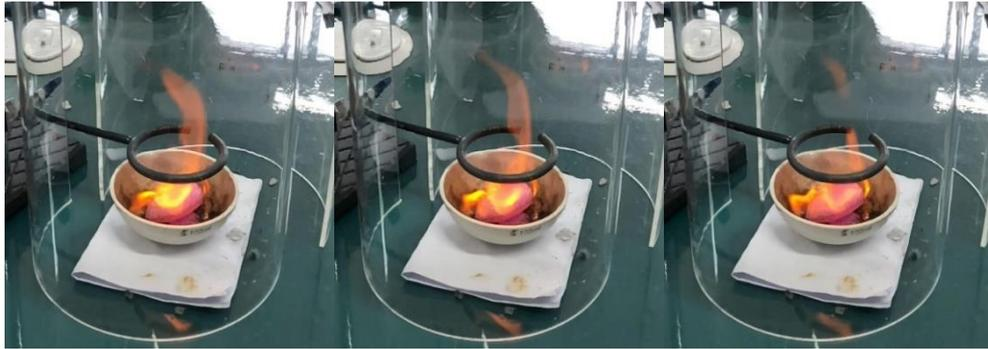
*Figure 3.4. The fire whirl is generated by solid alcohol, which is replaced by a 98% volume fraction of liquid alcohol in the following experiment.*
