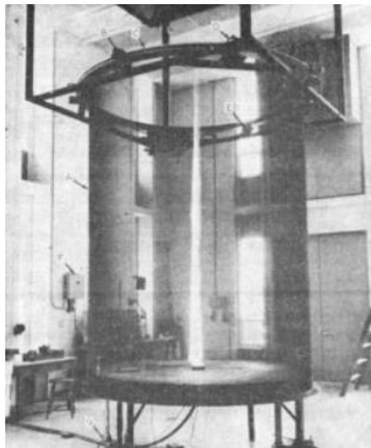
*Figure 2.30. A pool-fire-based off-source fire whirl generator[16].*
