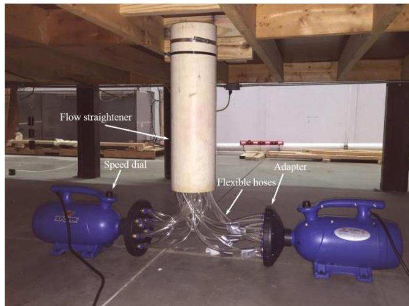
*Figure 2.14. The air jet is utilized in the firebrand transportation experimental [80].*
