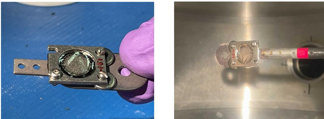
**Figure 4.8:** Images of the final targets that are being prepared to be irradiated by the  $^{14}\text{C}$  beam at ATLAS.
