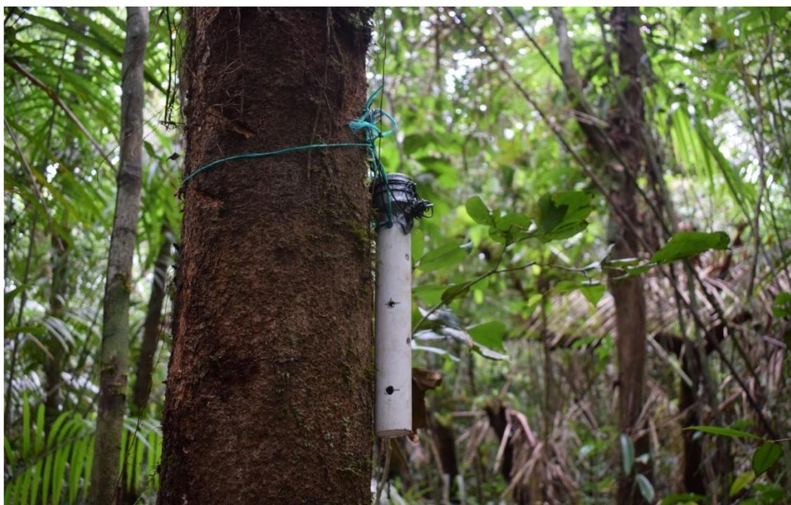
**Figure 4.3.** Example of a barologger attached to a tree trunk along the Lokolama transect. The plastic tube was capped with a tin can and duct tape. Photo by the author.
