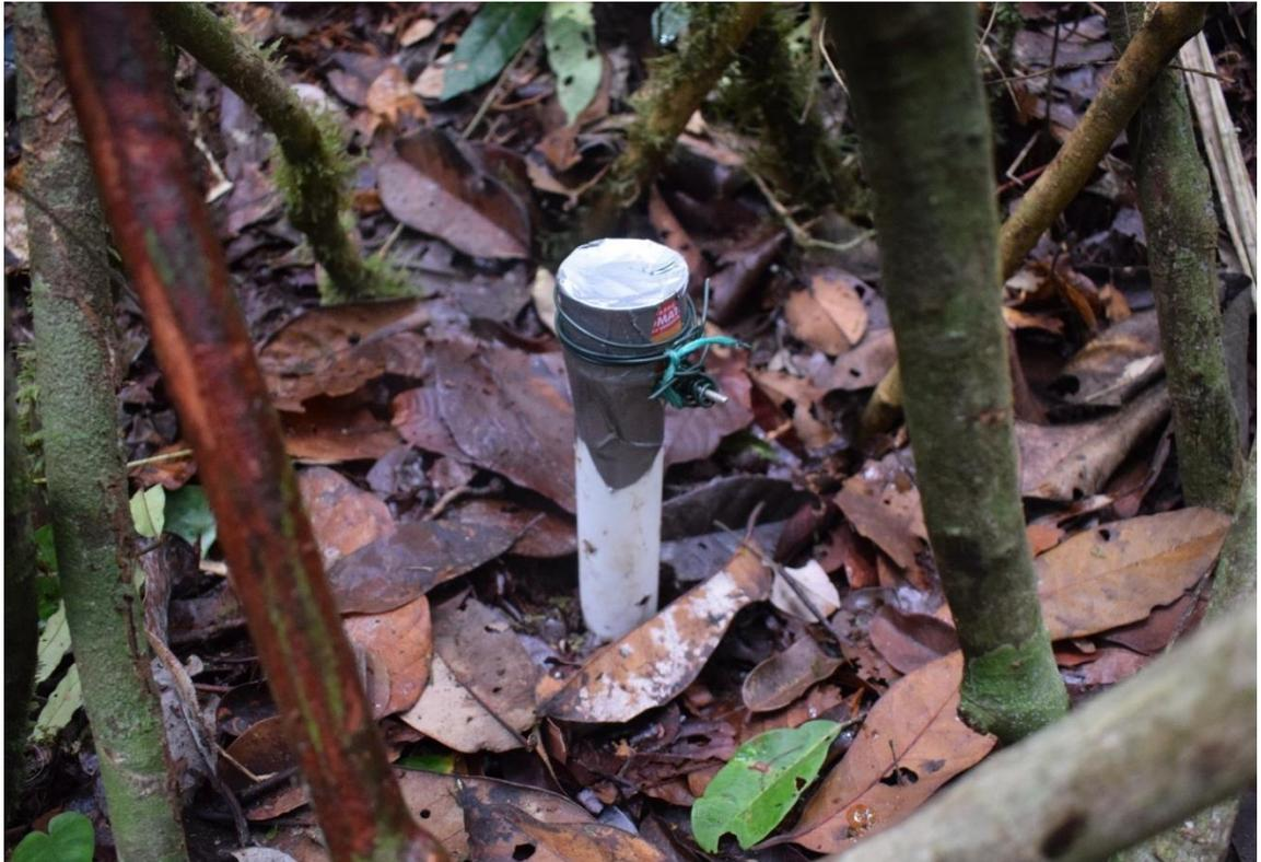
**Figure 4.2.** Example of a water pressure logger installed in the peat surface along the Lokolama transect. The plastic tube was capped with a tin can and duct tape. Sticks were placed around the tube to try to keep animals out. Photo by the author.
