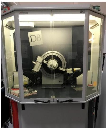
**Figure 3-11.** Bruker D8 Advance X-ray diffractometer (XRD) used in this study, LEMAS University of Leeds
