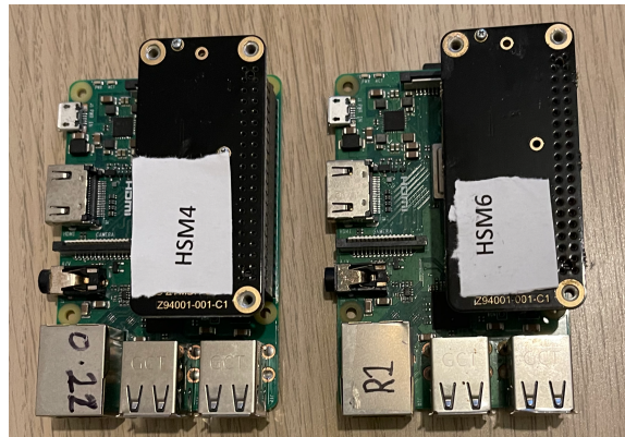
Figure 7.4: Two R-pis, one equipped with the HSM4 and another with the HSM6.
