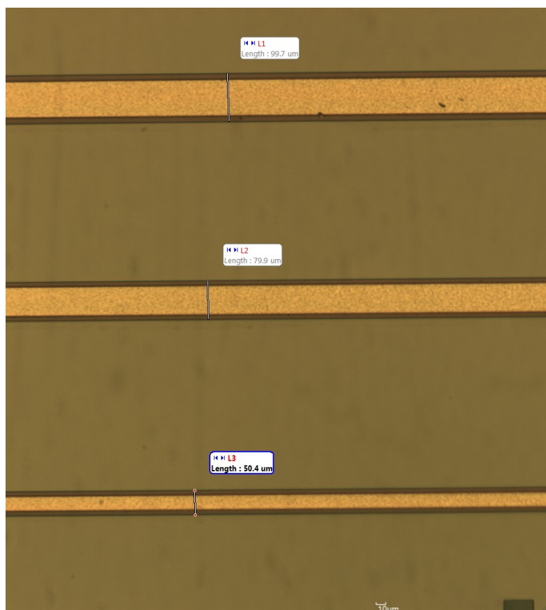
Fig 2. 2 Typical broad area laser fabricated with laser width of 100μm, 80μm, 50μm. The measured length is within the error of lithography.
