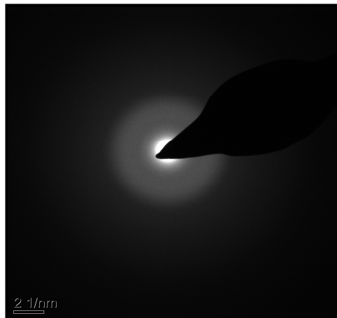
Figure 5-12 Diffraction pattern of PT glass-polymer composite thin films measured using TEM
