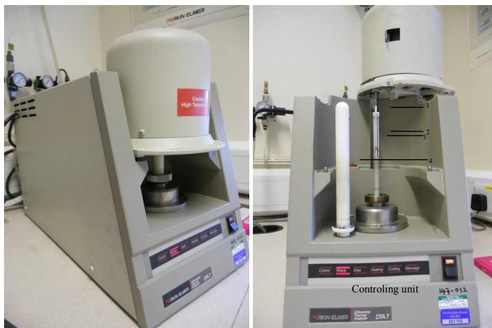
Figure 3-4 Setup of the DTA instrument. 1, purge tube, 2 and 3 are thermocouples for sample (left) and reference (right), respectively, and 4, protection tube
