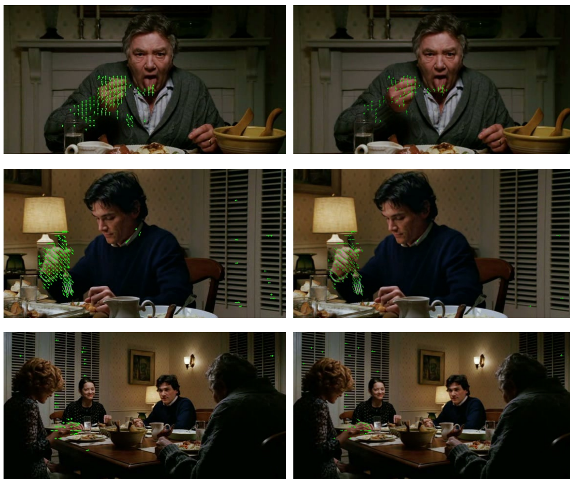
Figure 3.4: Side by side comparison of thresholded dense optical flow extracted with the Farneback OpenCV implementation with identical parameters at original (left) and 2\times scale (right). Arrows are plotted proportional in length to the magnitude of flow every 8 pixels in x and y directions at original scale and every 16 pixels at the double scale. Only flow with a euclidean magnitude greater than 2.5 (original scale) and 5 (double scale) is displayed.
