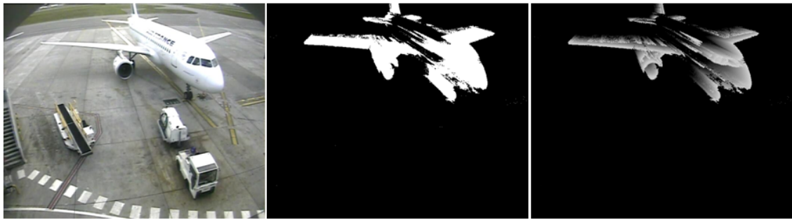
Figure 2.2: Illustration of MEI (centre) and MHI (right) for an aircraft arrival event taken from the cofriend dataset.
