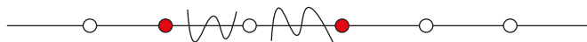
Figure 1: The classical repetition code of parameters [7, 1, 7] . Bits are placed on edges and checks are on circles. Each circle/check evaluates that the two edges incident to it have the same parity. Wiggly lines represent flip errors and red circles highlight the checks whose incident edges have different parity i.e. red circles represent the support of the syndrome. We note how flip errors on consecutive edges yield a weight two syndrome, with checks located at the boundaries of the error.
