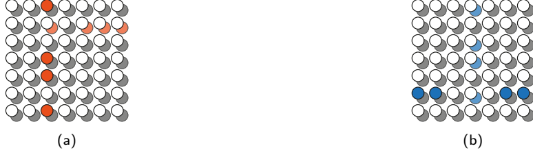
Figure 3: Graphical representation of the symmetric hamming code \text{HGP}_{\text{sy}}(H^T H) . In both figures, the left sector qubits sit at the front while the right sector qubits sit at the back. Sibling pair of qubits are superimposed. In fig. 3a the orange filled circles represent the support of the X stabiliser S_x(2, 3) . In fig. 3b the blue filled circles represent the support of the Z stabiliser S_z(4, 6) .
