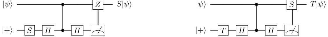
Figure 6: State injection gadgets for implementing S and T gates. The top wire in each circuit represents a logical qubit of a symmetric hypergraph product code and the bottom wire represents a logical qubit of an ancillary CSS code. To implement the CZ gates we use the pieceably fault-tolerant circuit in eq. (15). Note that for CSS codes the X basis measurements, represented as the gate H followed by Z basis measurements, can be done transversally.
