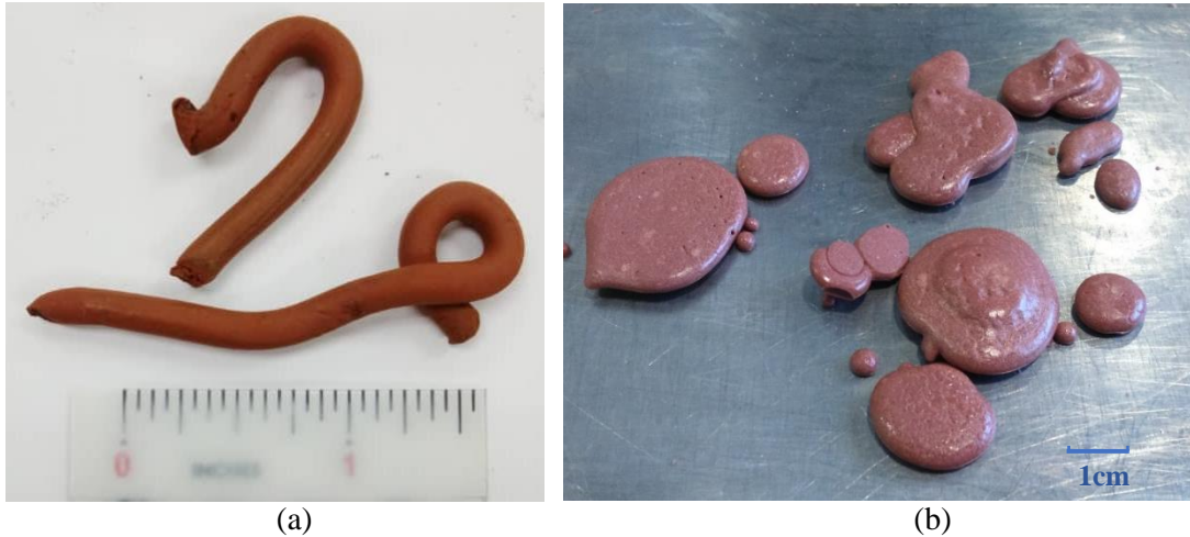
Figure 3.11; Examples of the physical form of extruded feedstocks at the pre-injection stage; (a) desired cylindrical shape of feedstock; (b) example of an unsuitable feedstock
