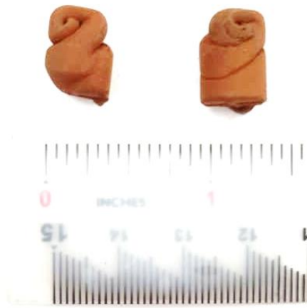
Figure 6.6; The green sample that does not completely fill up the mould and solidified
