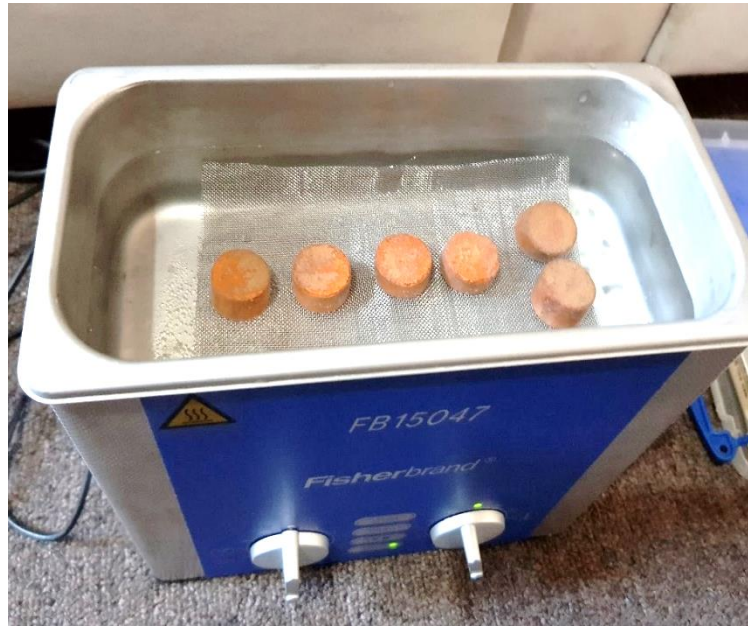
Figure 4.5; Water leaching process to remove KCl by using ultrasonic bath
