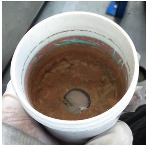
Figure 5.24; A hole at the bottom of the mixing container, caused by overheating from high energy generation with mixing media used
