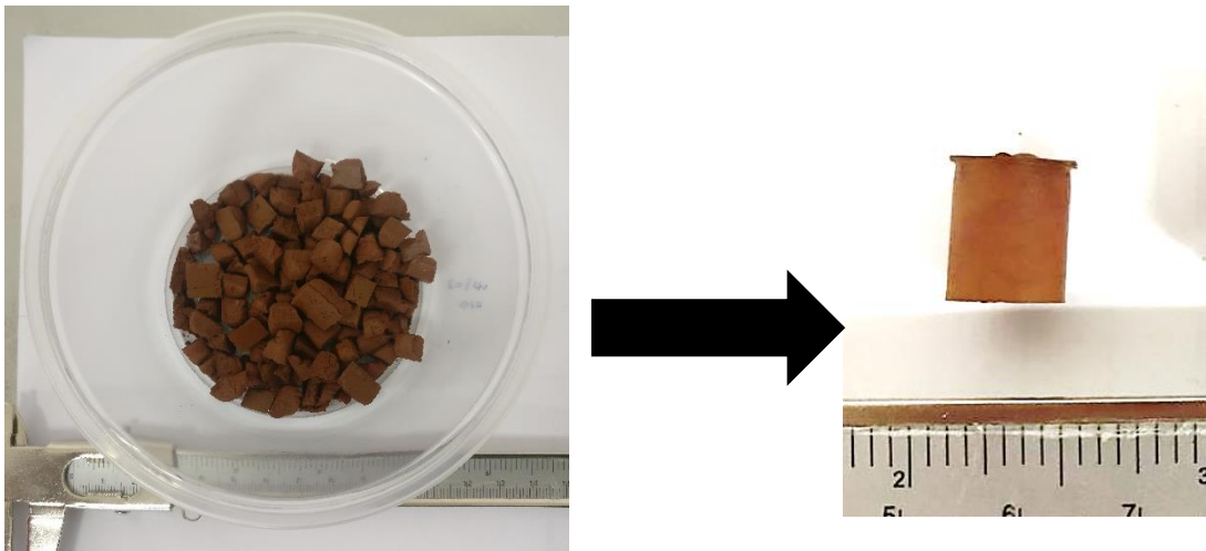
Figure 6.9; The transformation of feedstock into a green sample after the injection moulding process. The sample was made with 50% vol. KCl
