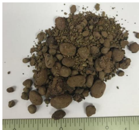
Figure 5.25; Defect samples obtained from the Multi-Phase Mode Mixing
