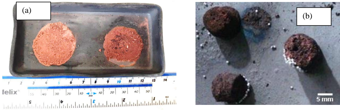
Figure 6.20; The poor-quality sample after the sintering process, a) The sample consists of too much PEG, b) The sintering was performed with high sintering temperature
