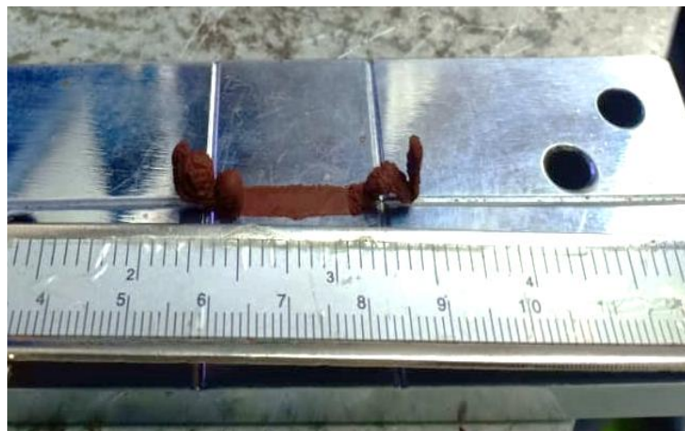
Figure 6.5; The feedstock 'stuck' at the inlet and cannot flow to the mould.
