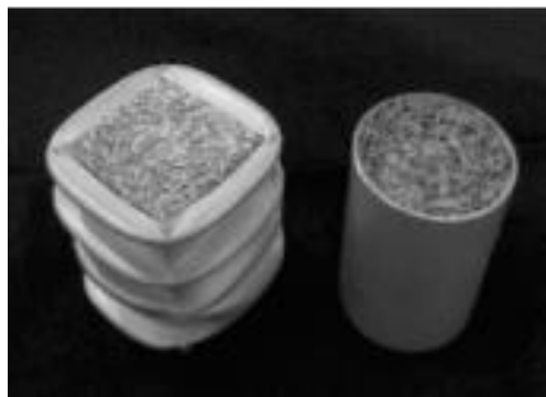
Figure 2.16; Prototypes of crash absorbers based on extruded aluminium hollow sections [70]
