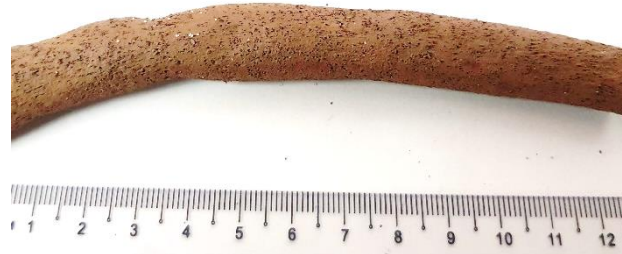
Figure 6.3; The Cu feedstock trapped inside the heated barrel.
