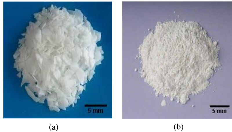
Figure 3.3; The current binders in solid form. (a) PEG 1500, (b) PMMA
