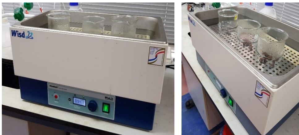
Figure 3.12; Water leaching process by water bath equipment, WiseBath WB
