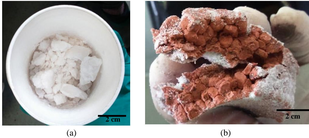
Figure 5.20; The investigation to find the optimum mixing speed and time to melt the binder. The process was carried out with a variation of speed and time (a) The binder was still in the solid state, (b) The shape of binder particles is clearly seen in the mixture of binder and powder (Cu, KCl)
