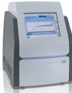
Figure 32 Roche LightCycler 96 instrument for RT-qPCR
