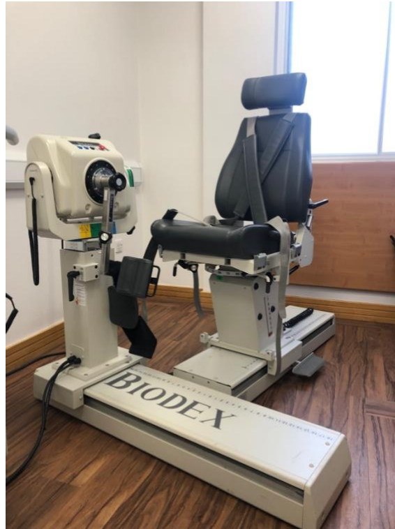
Figure 14 Biodesex System 4 Pro Dynamometer used for testing procedures in this study
