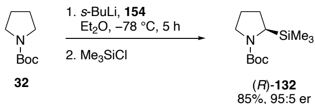
Scheme 3.14: (+)-Sparteine surrogate 154 mediated lithiation-trapping of N -Boc pyrrolidine 32
