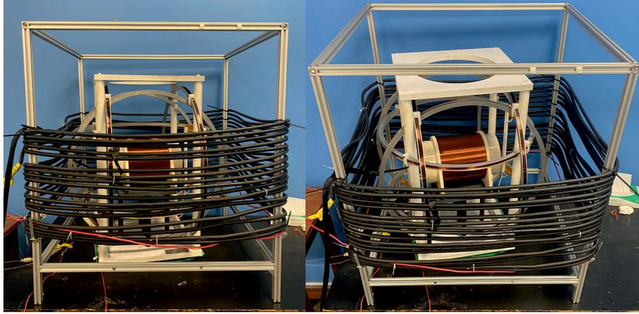
FIGURE 3.11: Image of the EFNMR-Helmholtz setup with a thick copper wire wrapped around it to block out electrical noise and improve the SNR of signals detected by the  $B^1$  coil.
