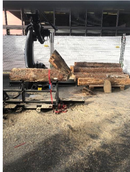
Figure 4.18 Robotic Chainsaw cutting working space
