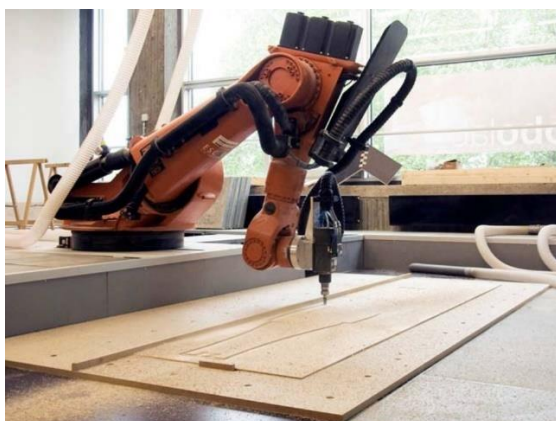
(a) Robotic milling on plywood strip
