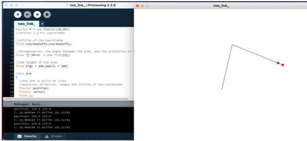
Figure 4.15 Two-link model built in processing
