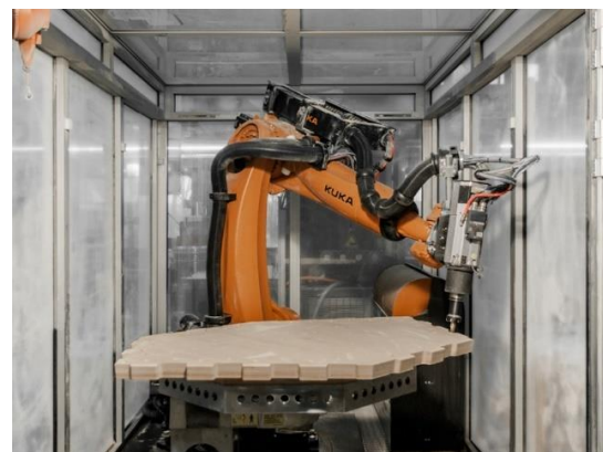
(b) Robotic milling on plywood plate
