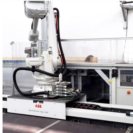
(c) The timber is gripped to the designated position for cutting
