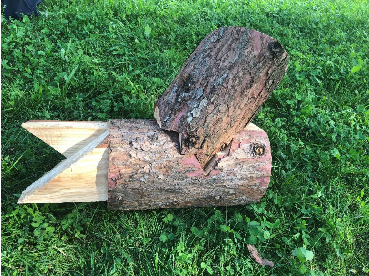
Figure 4.19 Wood joint cutting by the robotic chainsaw from the log
