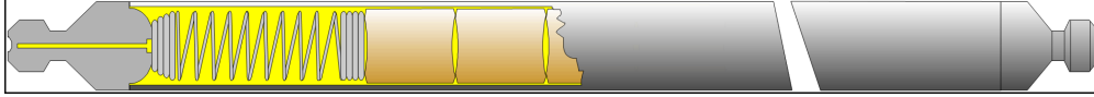
Figure 1.6: An outline of the internal structure of a fuel rod. This structure will be simplified for the conceptual model. Copyright National Nuclear Laboratory.
