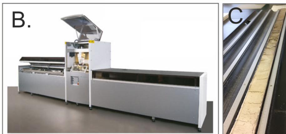
Figure 3.7-1. A) Schematic of ITRAX scanner instrumentation and main components. B) ITRAX Scanner similar to that housed at BOSCORF, with sensor housing and sample loader open. C) Example of an archive half barrel core.
