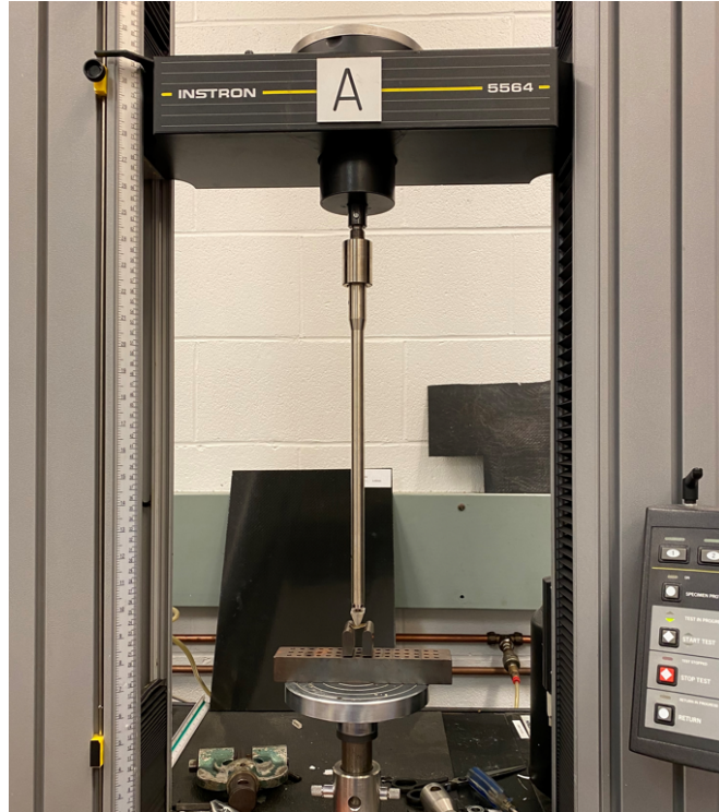
Figure 3.6: Apparatus set up for carrying out three-point bending tests in this project.
