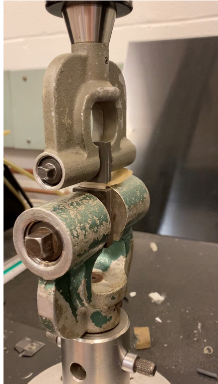
Figure 3.7: Apparatus set up for carrying out peel tests for determine peel strength of two layers woven all silk composites in this project.
