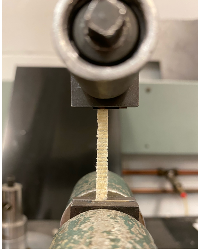
Figure 3.5: A piece of woven silk fabrics was gripped at two ends with small pieces of grinding paper, ready to conduct tensile testings.
