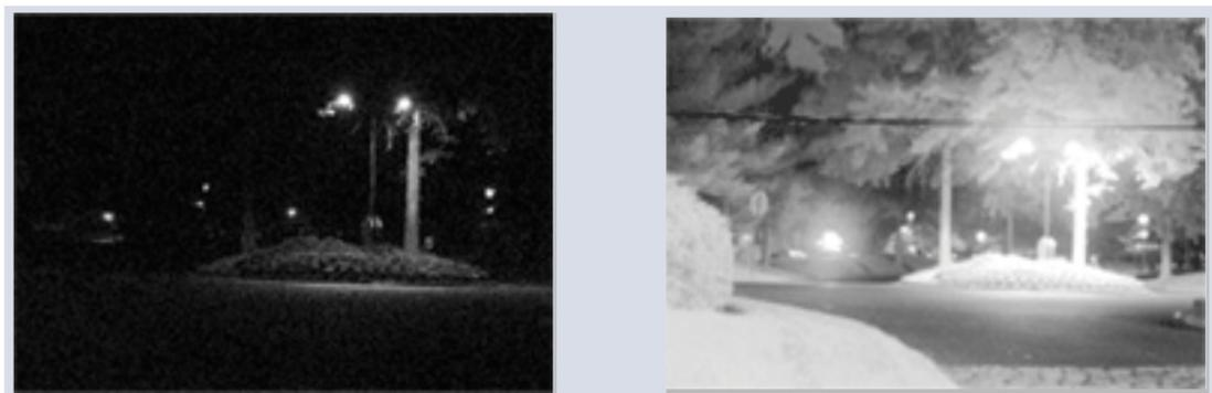
Figure 1.2 Comparison of the images taken from a visible (left) and SWIR (right) cameras at night [8].
