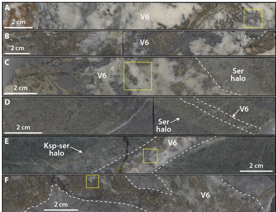
Figure 5.22. Representative V6 vein occurrences, from samples IC43-224 (A), IC37-218 (B), IC37-157 (C, D), IC01-052 (E) and IC33-030 (D). Sphalerite, chalcopyrite and pyrite dominate the ore mineral assemblage, with gangue minerals of quartz and carbonate. V6 veins make up most of the sample in A and B. Yellow boxes outline the approximate location of CL images in Figure 5.23.
