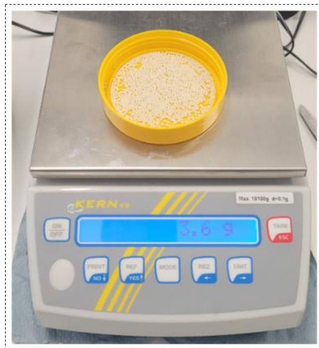
Figure 3. 30: 7.5% POM particles filling amount
