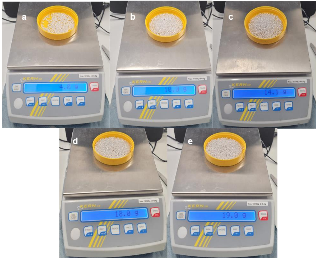
Figure 3. 26: Acrylic plastic filling amounts: Figure (a) is 10%, Figure (b) 25%, Figure (c) 35%, Figure (d) is 45% and Figure (e) is 47.5% filling amounts
