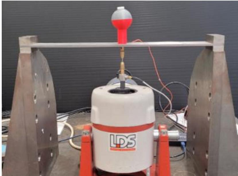
Figure 6. 12: Shaker-Beam-Individual resonator setup
