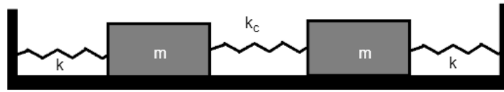
Figure 2. 10: Coupled mass-spring system example for tuned resonators
