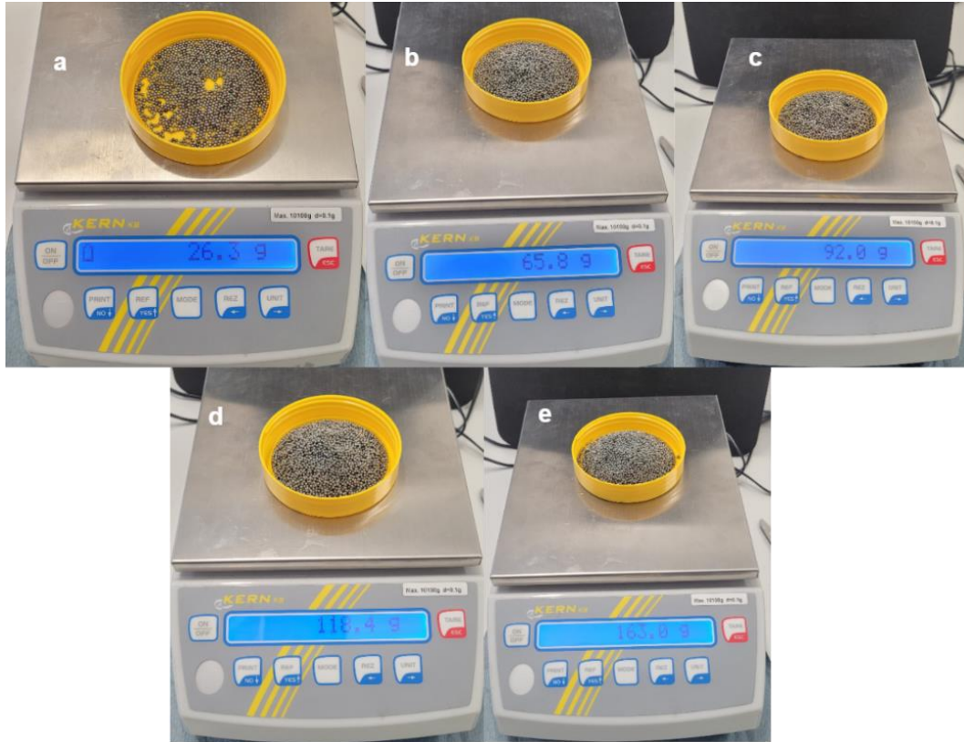
Figure 3. 22: Steel filling amounts: (a) is 10%, (b) 25%, (c) 35%, (d) is 45% and (e) is 62% filling amounts
