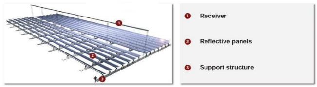
Figure 2-6: The LFR main components [49].
