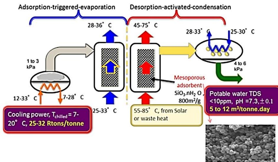
Figure 2-13: Schematic of the AD major components , illustrating the chilled and the potable water production using the available solar energy [84].
